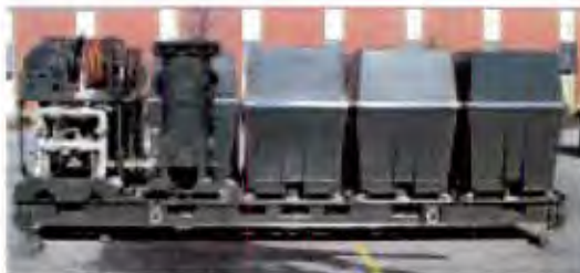
DMFD 400 with Pump and Filter/Separator Modules
