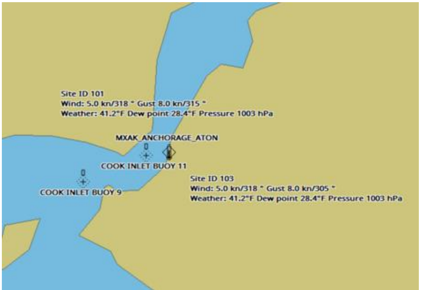
Figure 26. GateHouse Web GAD display of Virtual AtoN and Environmental ASMs.
