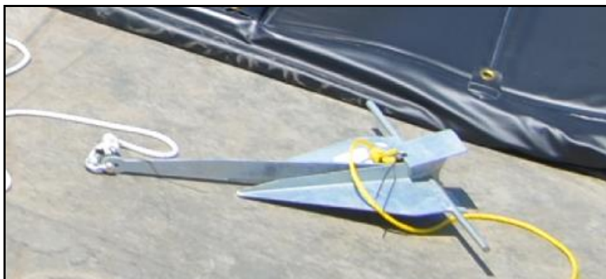
Figure 48. Improper anchoring method with the yellow buoy line that was corrected after the first deployment.
