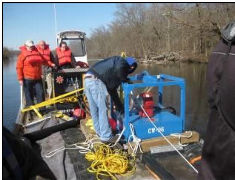
Figure 30. Hydraulic capstan (center) used to retrieve prototype back onto the barge.
