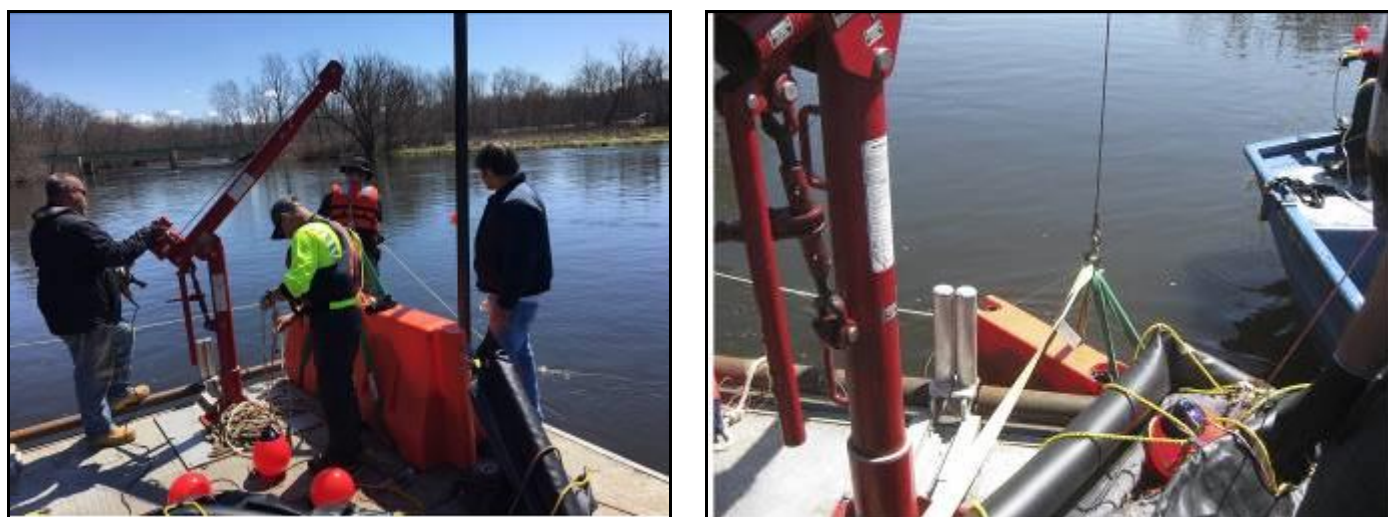
Figure 25. Inland mitigation system 1 prototype being deployed with barge's davit crane.
