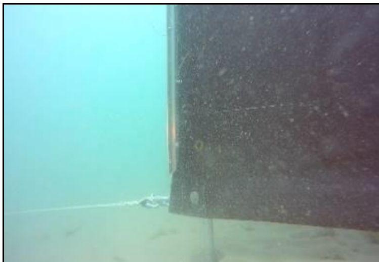
Figure 50. Tension of anchor line lifted the end of the mitigation system slightly.
