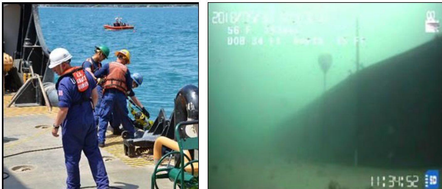
Figure 42. USCGC Hollyhock crew deploying a ROV (left), ROV image of mitigation system on the lake bottom (right).
