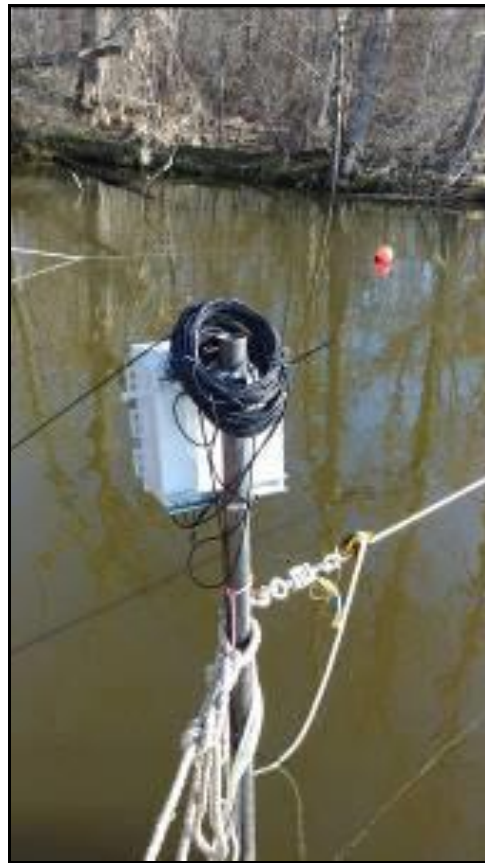
Figure 20. Data Acquisition System attached to anchor post on upstream side to collect tension data from load cells.
