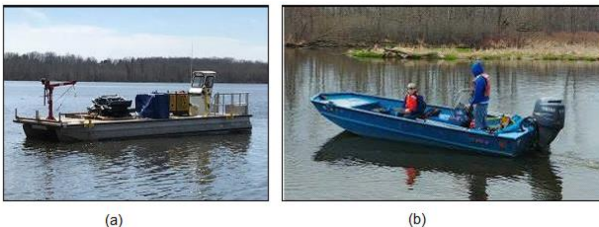
Figure 16. (a) 38 foot barge for deployment/retrieval operations and (b) 20 foot jet-outboard boat for supporting operations.
