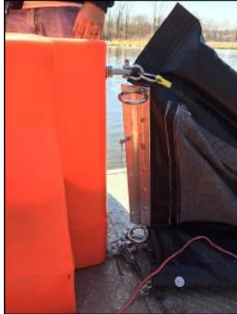
Figure 18. Jersey barrier connected to the inland mitigation system 1 prototype.
