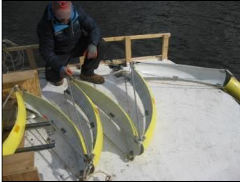
Figure 33. CLAMShell mitigation system being deployed into the Kalamazoo River.
