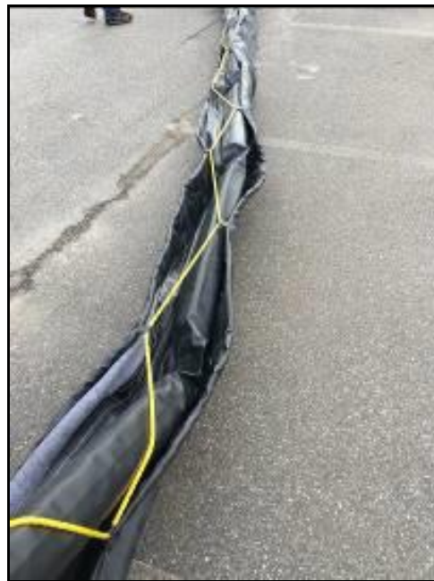
Figure 19. Compressed inland mitigation system with the scour flaps up and tied with a truss line.
