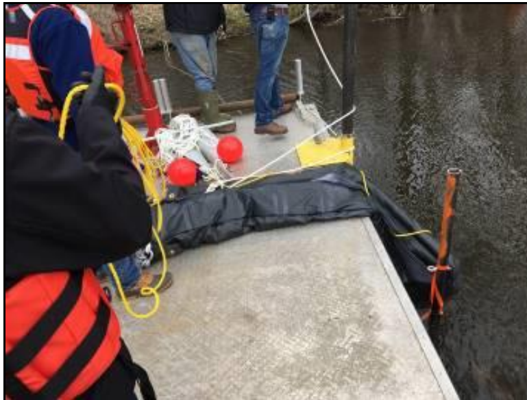
Figure 22. Inland mitigation system 1 prototype continues to be deployed on upstream side of anchor posts.
