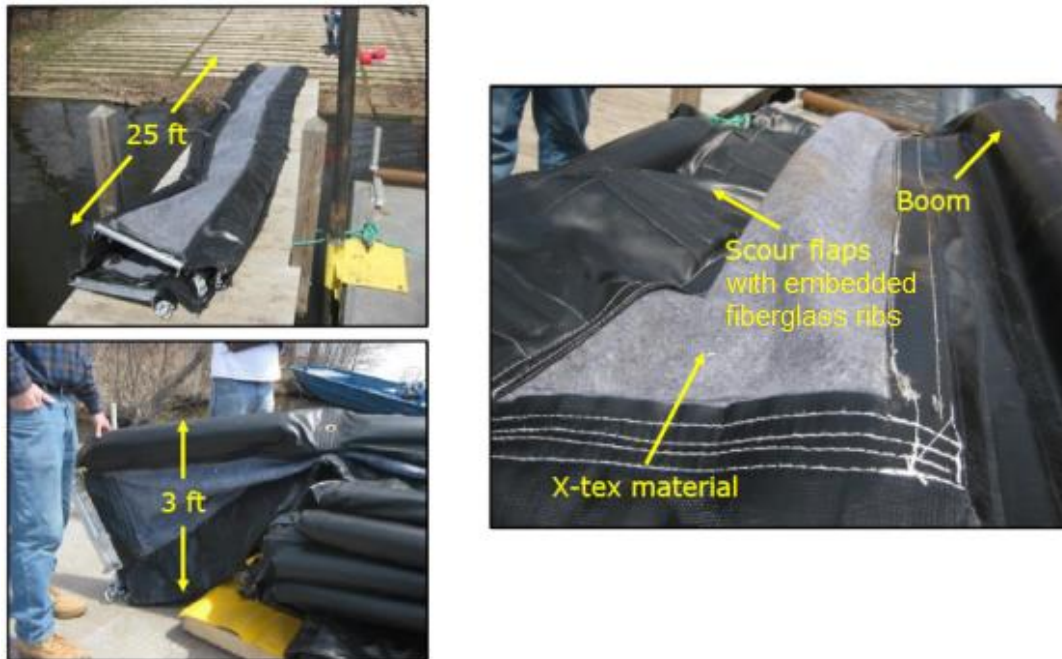
Figure 3. Inland mitigation system 1 prototype.
