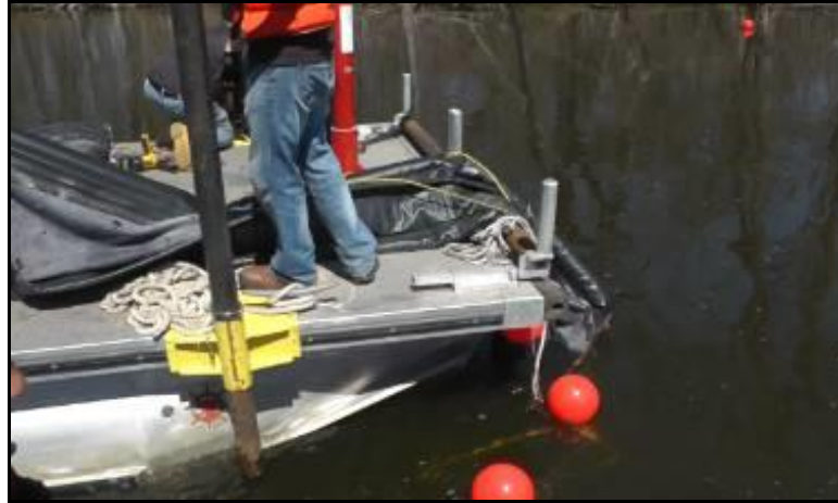
Figure 26. Inland mitigation system 1 prototype being deployed off the bow of the barge.
