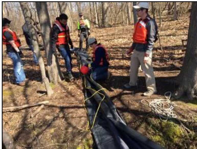
Figure 27. Compressing one section of the inland mitigation system 1 prototype with the truss line.
