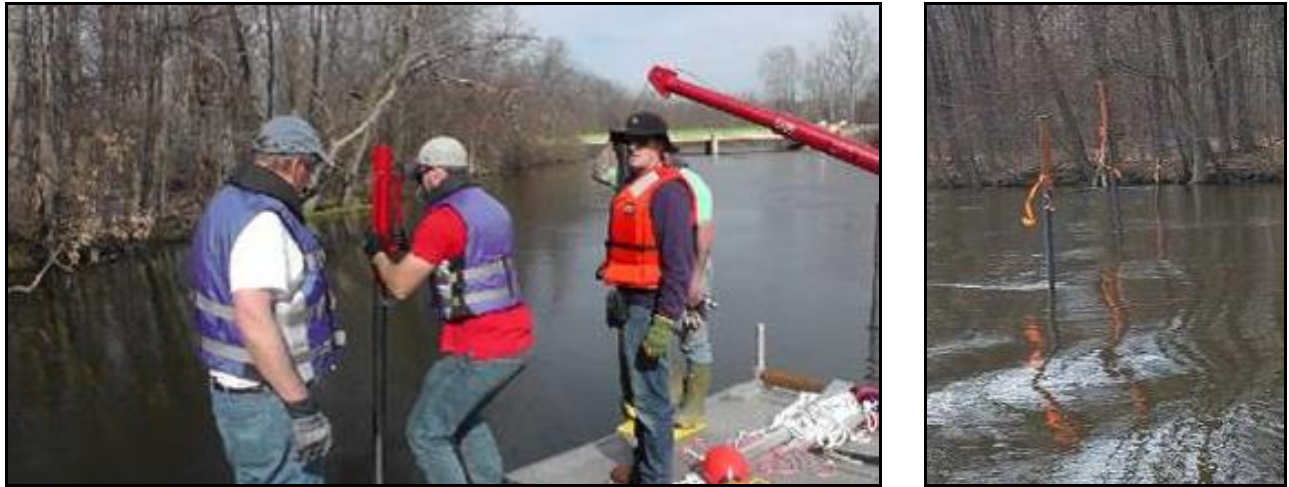
Figure 17. Three anchor posts driven into the Kalamazoo River in advance of the shallow water deployment test run.
