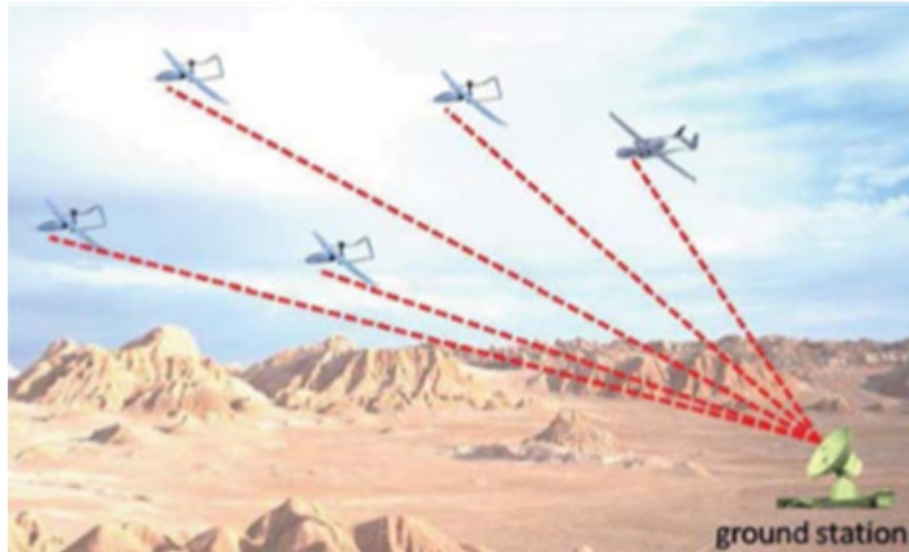
Figure 3. Centralized UAV Network Architecture. Source: Li, Zhou, and Lamont (2013).
