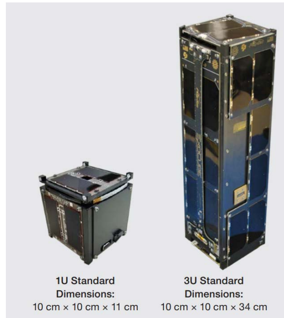
Figure 1. CubeSat Dimensions. Source: NASA (2017).
