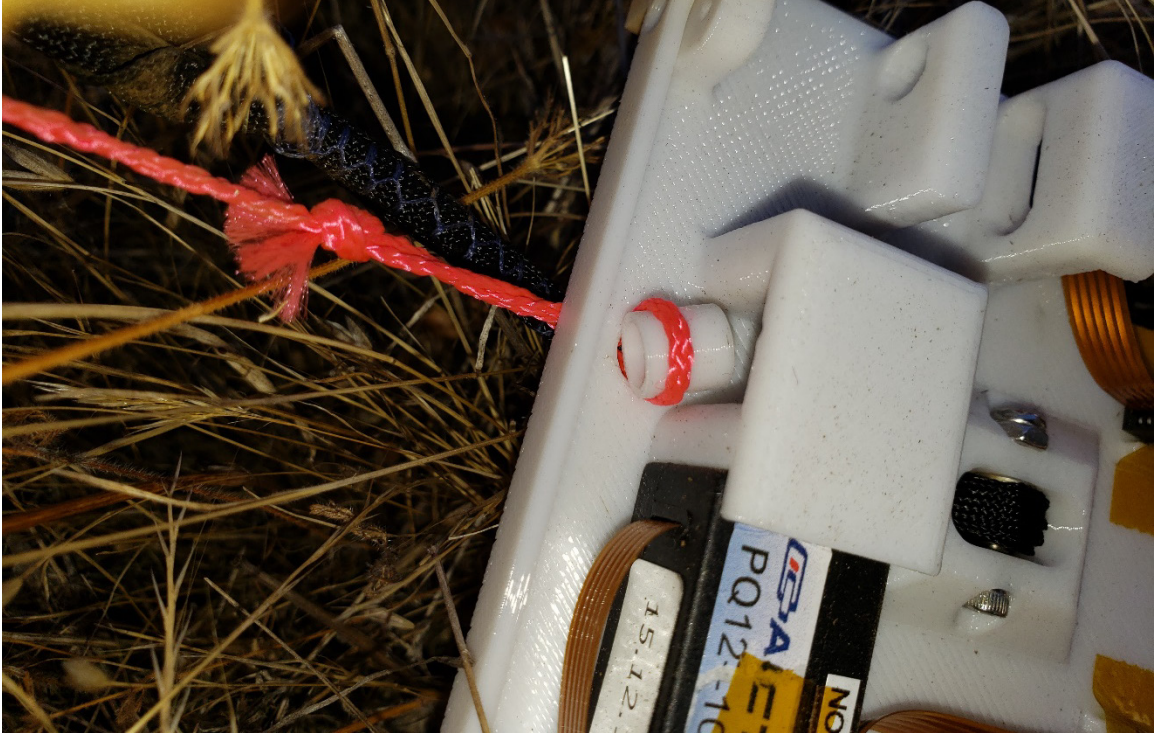
Figure 38. Balloon harness line and actuator sleeve caught on CubeSat frame
