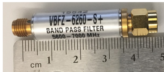
Figure 22. Local oscillator filter: Mini-Circuits VBFZ-6260-S+
