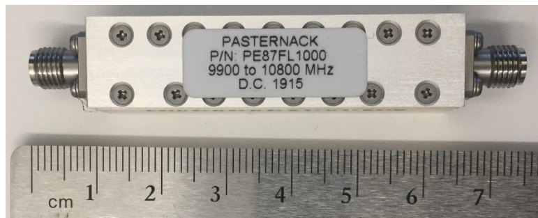
Figure 20. 10 GHz final bandpass filter: Pasternack PE87LF1000
