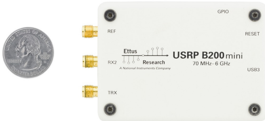
Figure 9. Ettus B200 enclosure compared with a U.S. quarter. Source [23].
