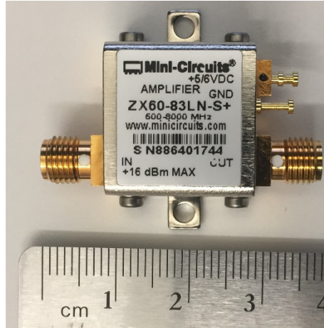
Figure 18. Intermediate frequency and local oscillator amplifiers: Mini-Circuits ZX60-83LN-S+
