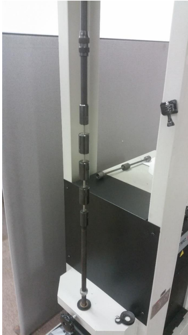
Figure 3: Sustained Load Test Frame
