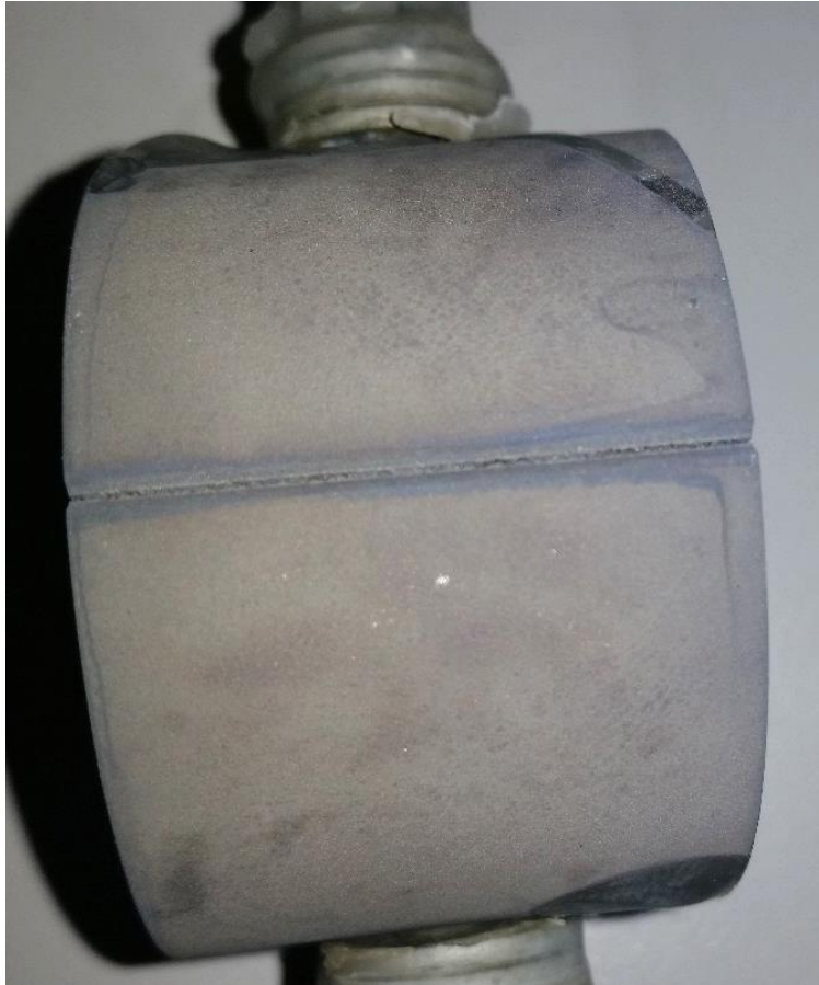
Figure 28: Coupon That Fractured During Plating
