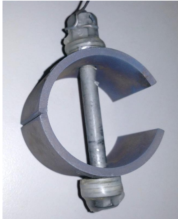
Figure 27: Coupon Electroplated Under Stress
