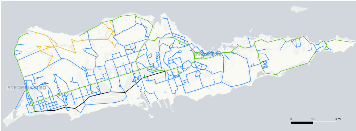
Figure 3.5. Arcs representing surface road network on St. Croix. Yellow lines represent dirt roads. Green lines represent rural roads. Blue lines represent urban roads. Black lines represent highways. Created using QGIS Development Team (2019) on 12 August 2019.
