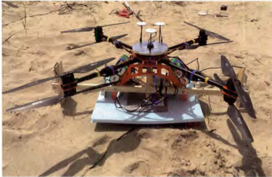
Figure 52 Bergen Quad 8 with radar and array antennas attached ready for flight
