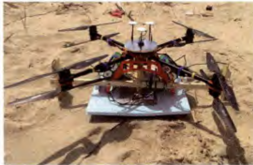
Figure 1. Bergen Quad 8 with radar and array antennas attached ready for flight.
