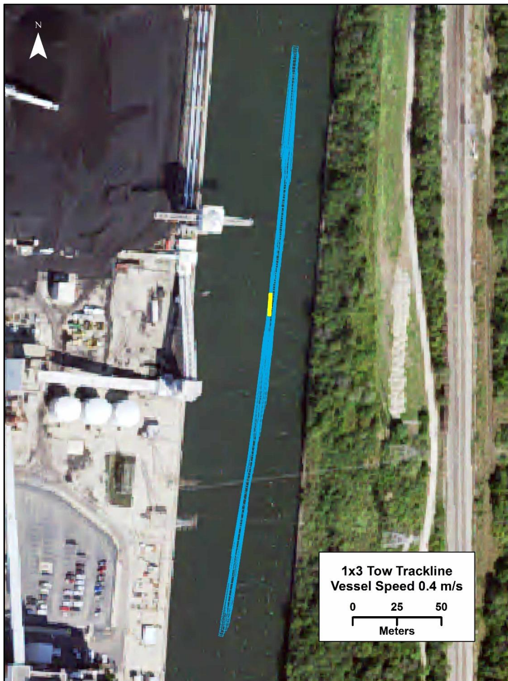
Figure 4-2. Vessel tracks indicating the off-center approach to the jets. The yellow rectangle denotes the approximate profile of the jet manifold.
