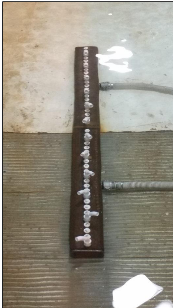
Figure 6-1. Manifold configuration for successful jet tests in the laboratory. The barge approaches from the top of the photograph. The nozzle angle increases in an alternating pattern along the manifold axis, thereby directing the flow farther from the centerline of the barge as it passes over the array.
