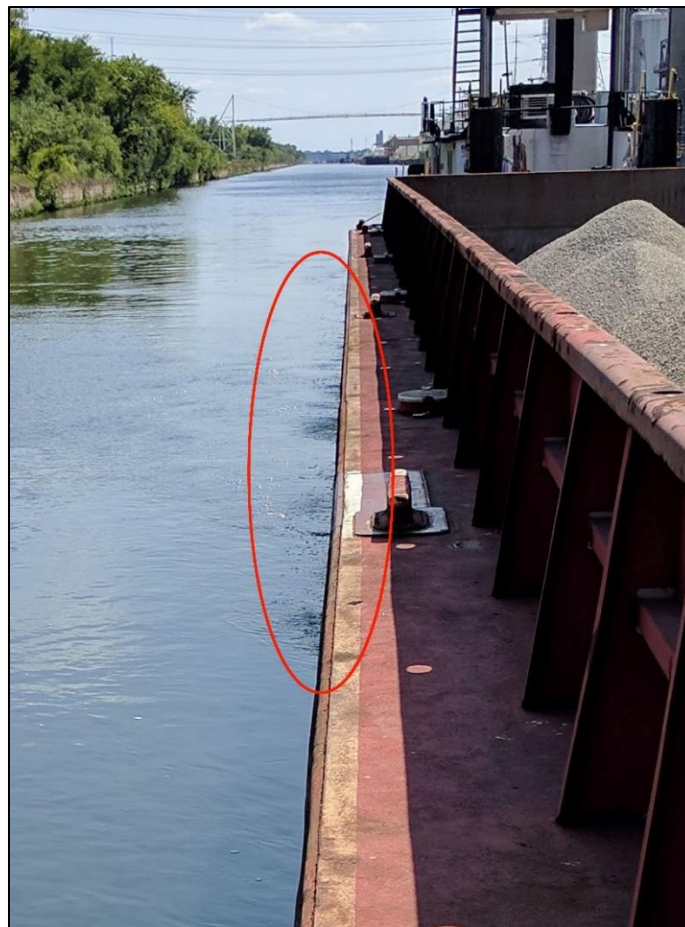
Figure 6-3. Photograph depicting air bubbles issuing from beneath the barge. Bubbles were seen rising to the surface along the hull for several minutes after the tow had cleared the manifold.
