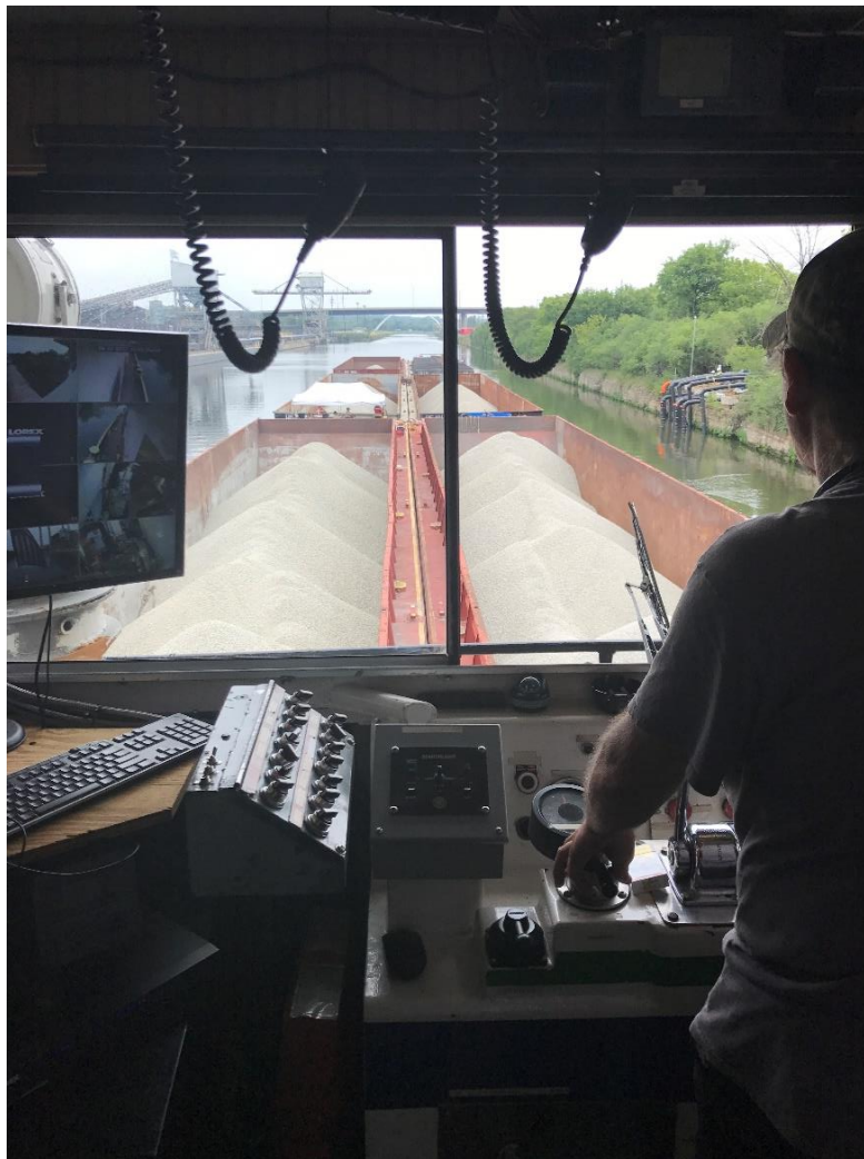
Figure 3-6. View from the wheelhouse of the MV Derek E showing the 2 \times 3 barge configuration. The leading barge is about to pass over the manifold.
