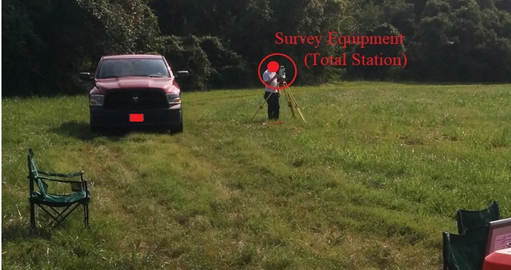
Fig. 25 Swarm RF relative localization survey equipment (Leica TS16 Robotic Total Station) that records known positions in the (X,Y,Z) dimensions
