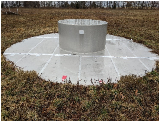
Fig. 27 a) Photograph of the metal tophat reflector present at Webster Field during the deployments. The height of the central cylinder is approximately 1 m.
