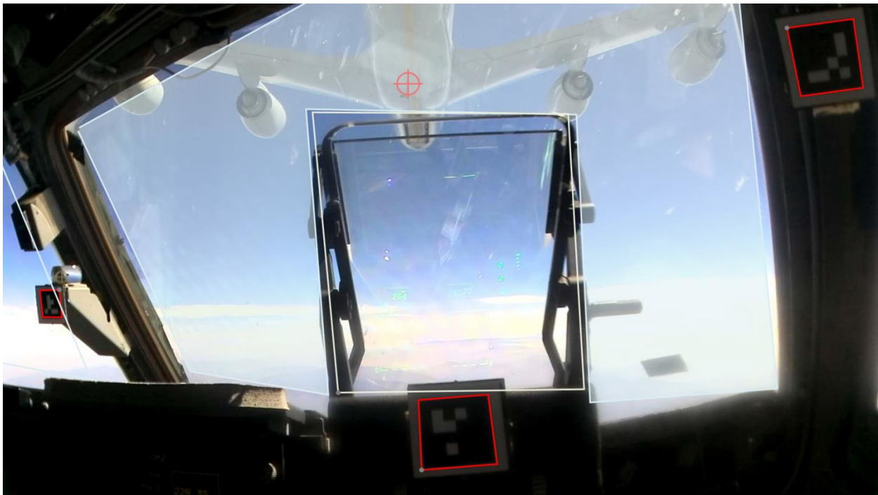
Figure 32: Eye-tracker scene camera view during aerial refueling task
