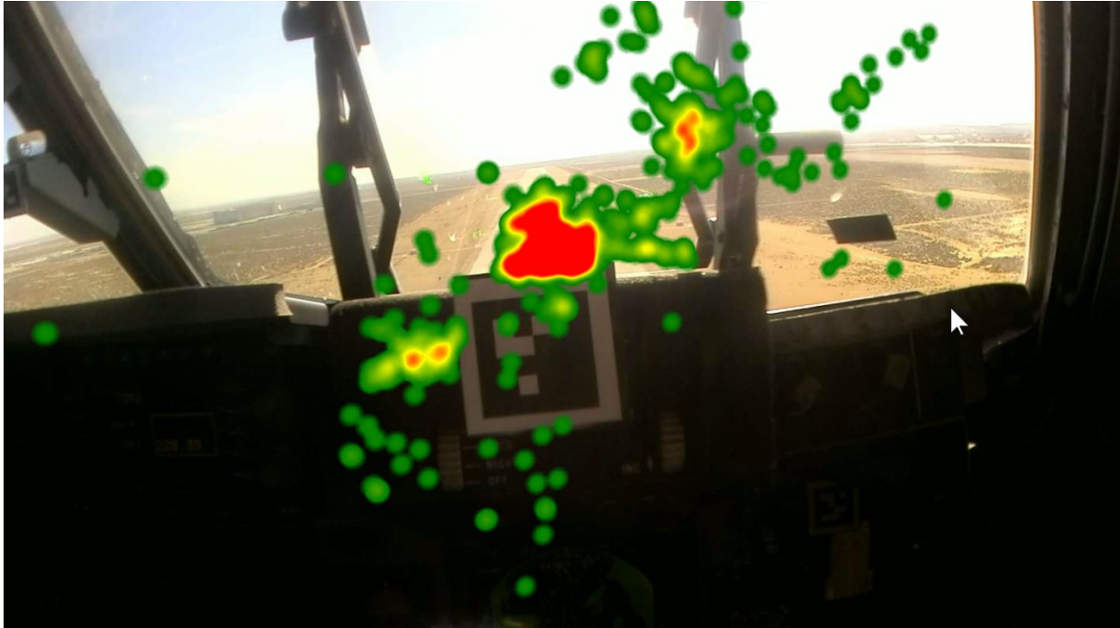
Figure 37: Heat map showing which areas the current pilot most frequently focused on during Landing
