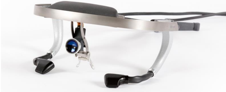
Figure 6: Dikablis Professional Glasses (photo from Ergoneers, Inc.)
