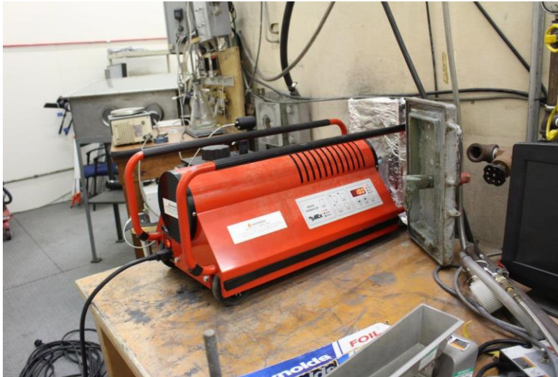
Figure 8. Smoke generator outside the chamber with a nozzle inserted into the access port.
