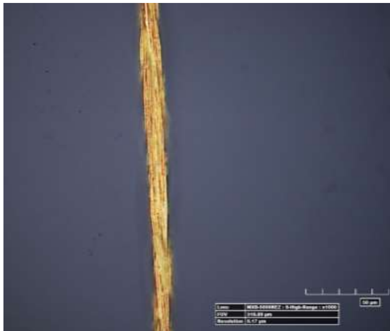
Figure 59. Optical image of a twist of 5 bundles of 5 ALD insulated nanowires (25 wires total)
