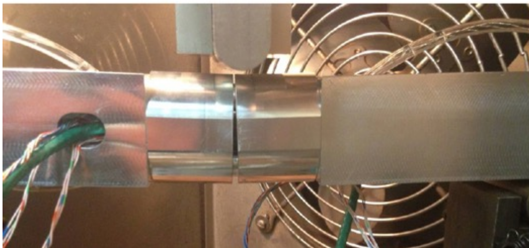
Figure 45. Connector Torque Testing (Three Point Bend)
