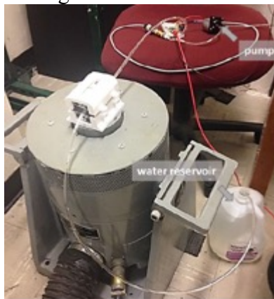
Figure 51. Fluid System Used for Vibration Testing
