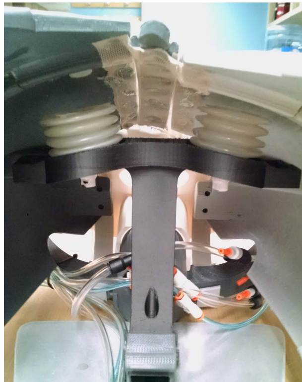
Figure 38. Chest rise actuation bellows with support and displacement sensor mounting locations; rib cage with floating sternum
