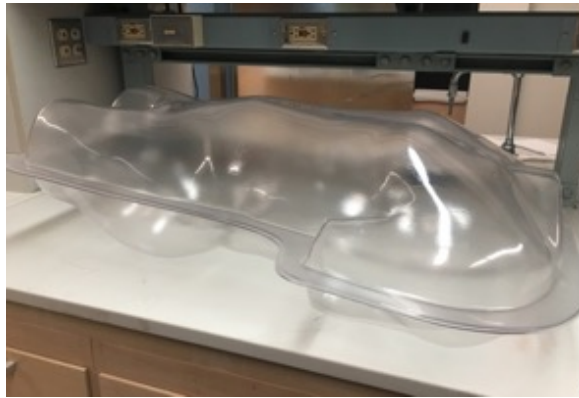
Figure 11a. Mold castings from model Figure 11b. Hollow thermo-formed manikin shell
