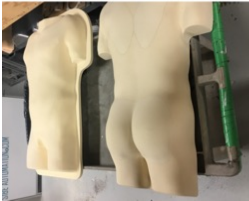
Figure 11a. Mold castings from model Figure 11b. Hollow thermo-formed manikin shell
