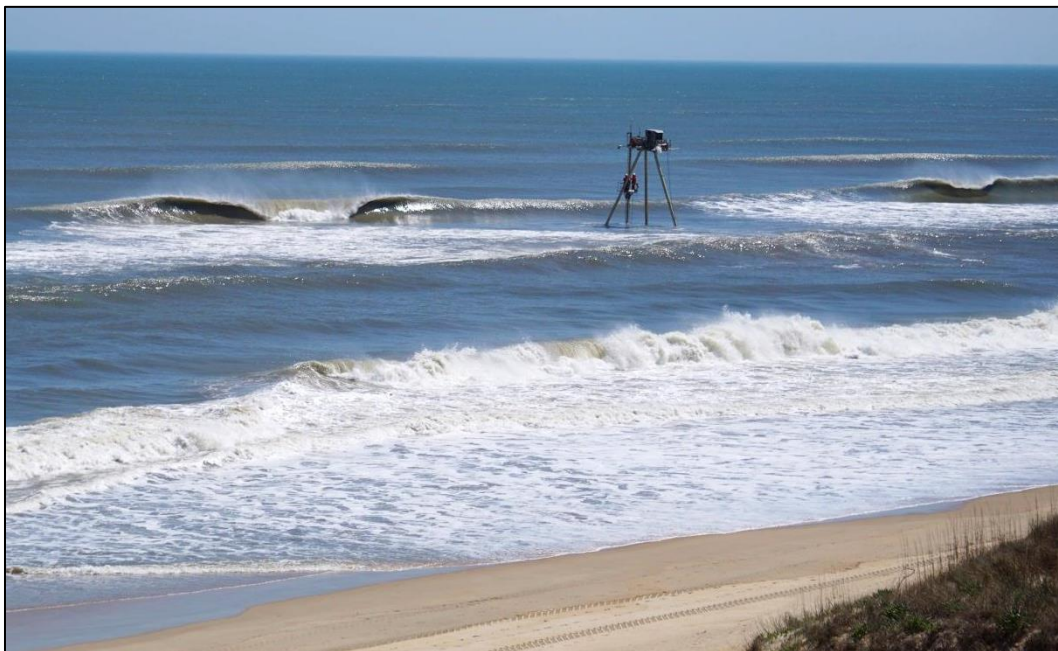
Figure 5. CRAB sampling at or just inshore of the breakpoint during plunging breakers on 04 April 2017.
