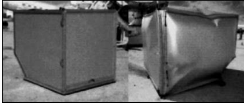
Figure 7: ECOS-3 Blast Resistant Cargo Container Before and After Blast[16]
