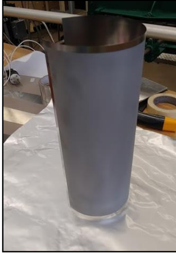
Figure 50: Deformed foil after single side grit-blast
