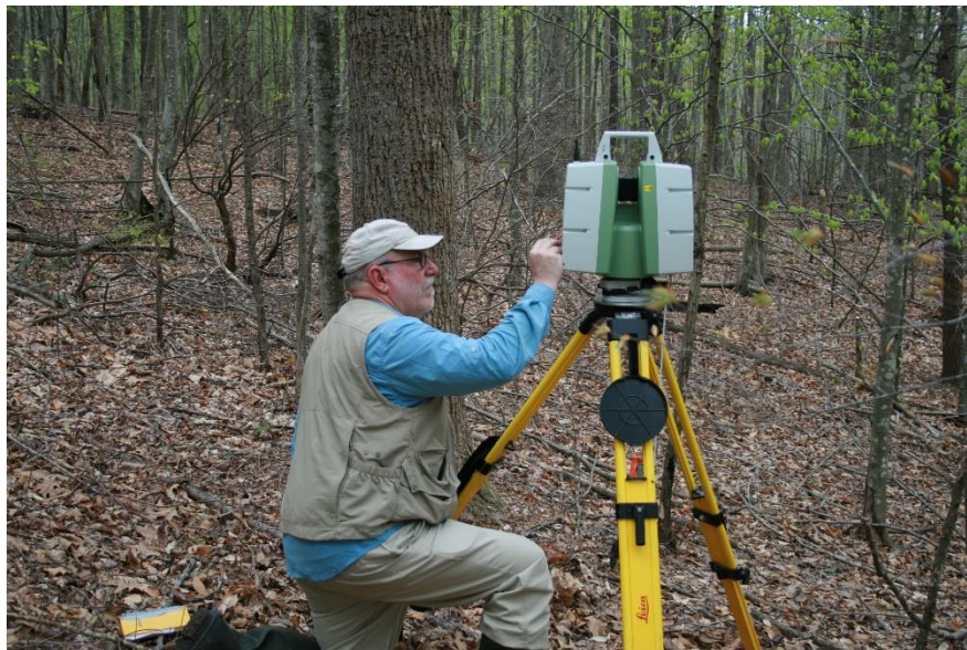
Figure 1. Leica C10 Terrestrial LiDAR scanner setup.
