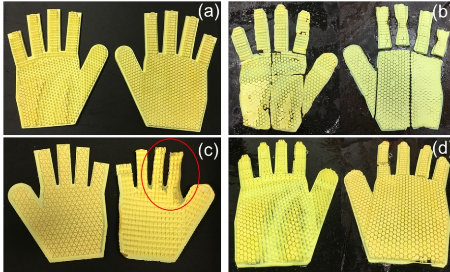
Figure 5. Aerogel tiles made of Airloy ® X116: (a) a set of tiles fabricated by Molding & Casting and supercritical CO 2 drying process, (b) a set of tiles from (a) glued to the elastic backing fabric showing various defects caused by polishing and gluing, (c) a set of tiles fabricated by Machine Slitting – the area damaged by oil drips is indicated by a red circle, and (d) a pair of tiles ready for the fabrication of the Polar Grip Revision 5 after Molding & Casting, ambient drying, polishing, and gluing.
