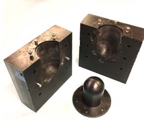
Figure 24. Mold for Manufacturing the Rubber Housing for the Underwater Operation. Source: [5].
