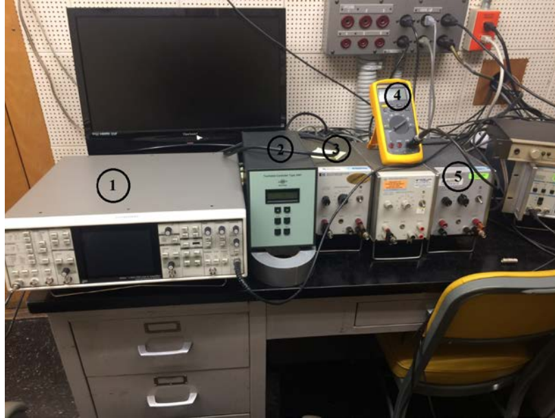
The figure shows the set-up and controls for performing the tests in the anechoic chamber. 1. SR865 lock-in amplifier 2. B&K Type 5997 turntable controls 3. Back-up HP467A power amplifier 4. Multimeter 5. HP467A power amplifier.
