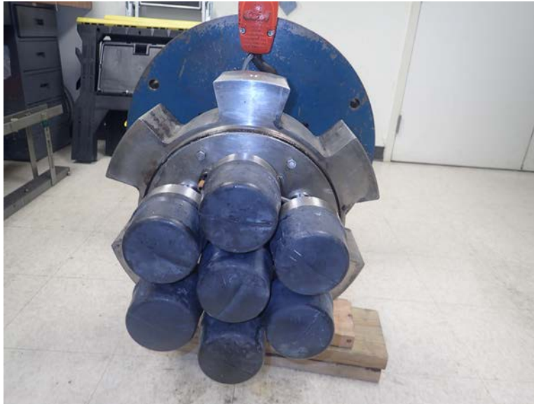
Figure 32. Sound Source Located at Each End of System L Test Vessel
