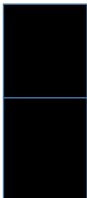
Figure [2] Depicted here are two pixels. Both pixels here are in the “off” state, and so in matrix notation, the pixel values would yield zero.
