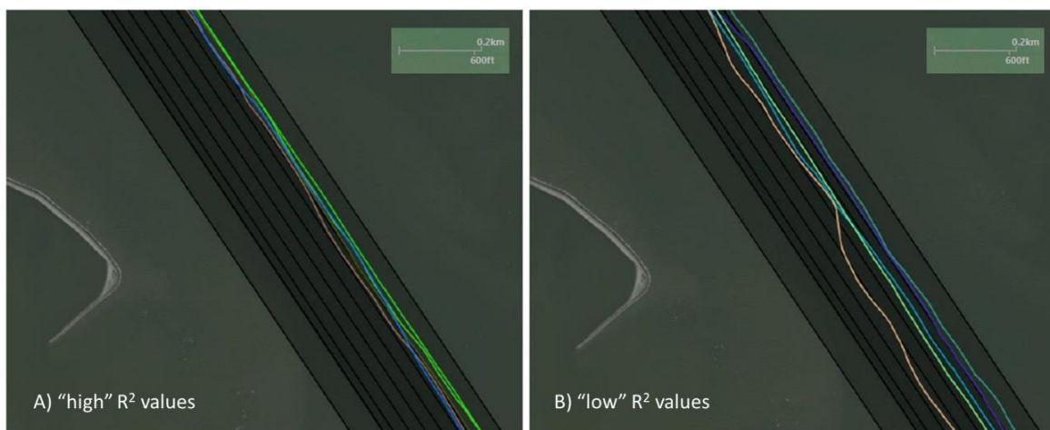
Figure 11. Comparison of towing vessel tracks with relatively high R^2 (panel A) and low R^2 (panel B) coefficients within a southern portion of HSC-S2.
