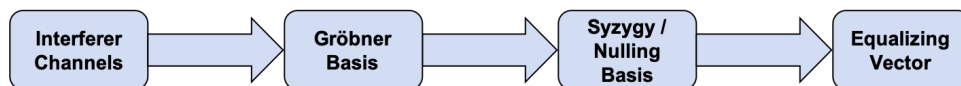
Figure 24. The interference channel matrix is first converted to a module Groebner basis. The combinations of rows of the channel matrix that zero-force are computed from the coefficients used to form the Groebner basis. This provides generators for all zero-forcing weights. If required, the zero-forcing generators are applied to the array response of the desired signal. The resulting Ore polynomials generate a left ideal whose Groebner basis is evaluated. If the ideal contains a monomial, equalization is possible.
