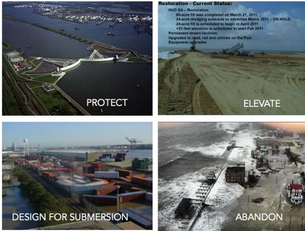
Figure 1. Four levels of port adaptation strategies: Protect, Elevate, Design for Submersion, and Abandon (Images: Protect, photo by www.dutchwatersector.com ; Elevate, author unknown; Design for Submersion, Alabama State Port Authority; Abandon, Dan Cuellar 2012.)
