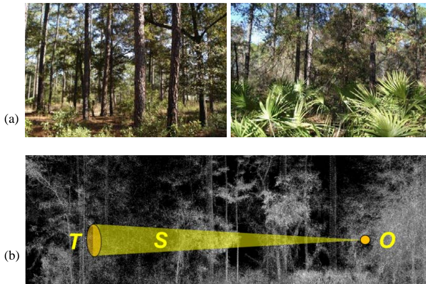
Figure 1. (a) Photos illustrating general scenes about the study areas for Site 1 (left) and Site 2 (right). (b) Concept of a BC-LOSV scope function, S , between the observer, O , and the target, T , showing terrestrial lidar points.
