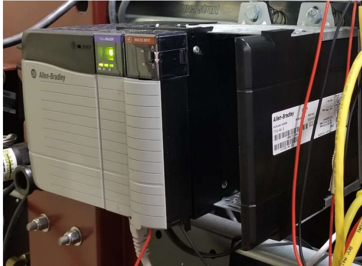
Figure 21. PLC with Ethernet/IP and Analog Modules.
