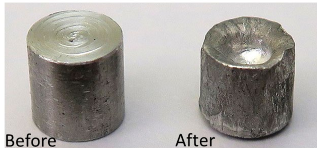
Fig. 4 Aluminum projectile prior and after launch; image shows cratering occurs at the back of the soft-captured pellet
