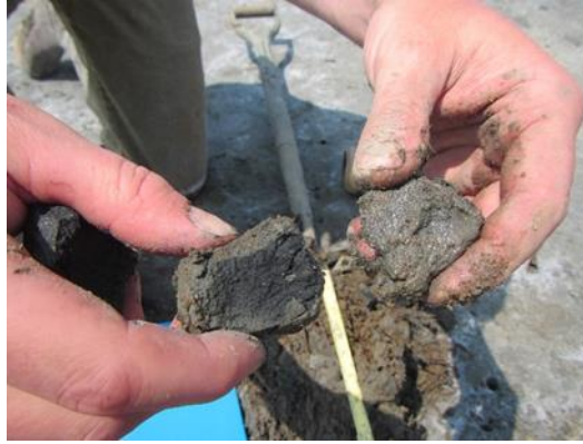
Figure 5. Dark soil coatings (soil on left) from iron sulfide soil materials at Avalon, then oxidized with 3% hydrogen peroxide (soil on right) resulting in removal of dark soil coating and revealing of the underlying grey soil matrix color.
