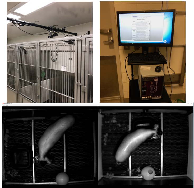
Fig. 5. Pig Epilepsy Monitoring Unit (EMU). Images above demonstrate the video acquisition using IR for 24 hour recordings/monitoring of the pigs (2 shown). Also depicted is the acquisition system for the wireless data, as well as the home cage with the IR illuminators, cameras, and wireless hubs.
