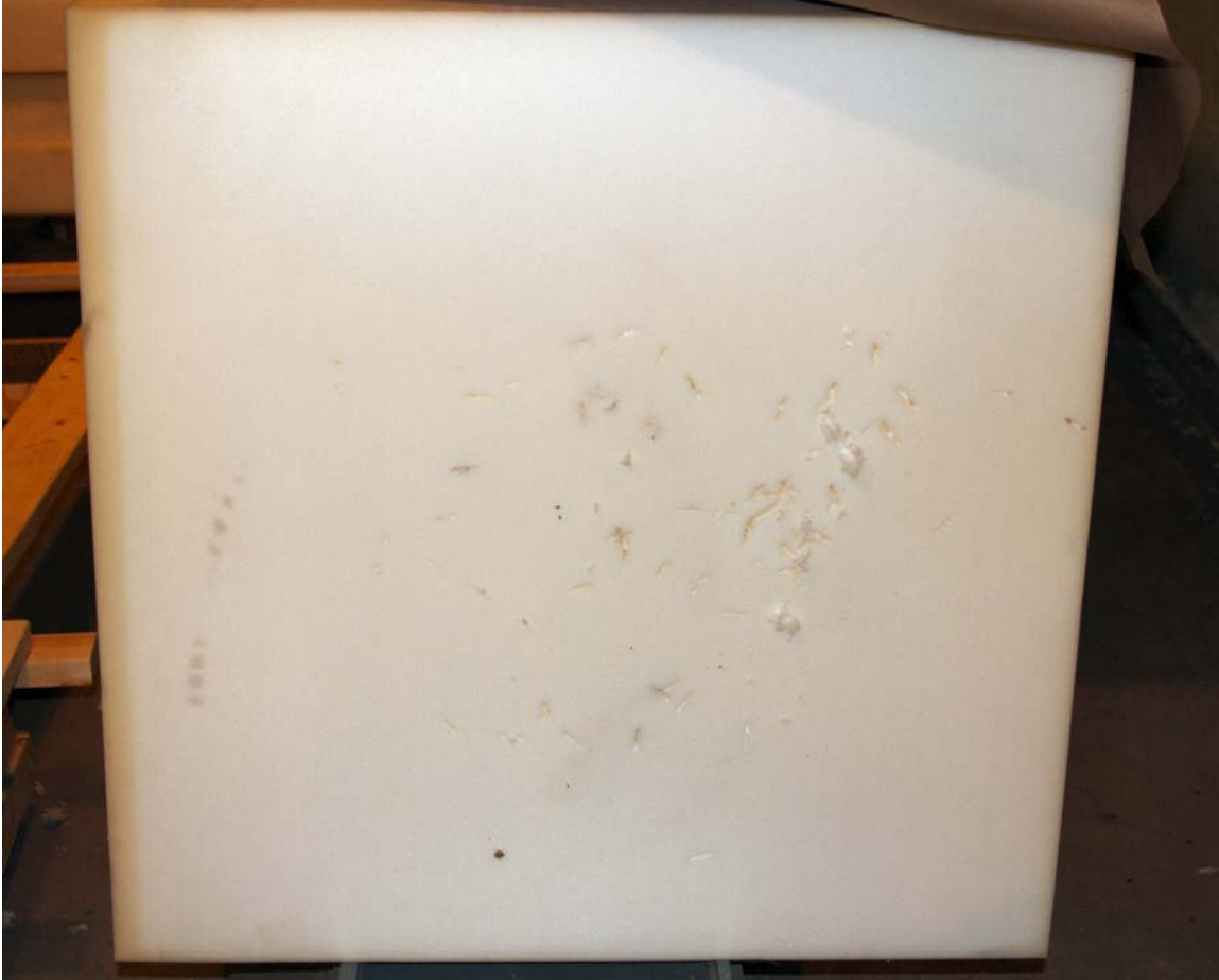
Figure 5. Foam block showing minimal damage from multiple impacts.
