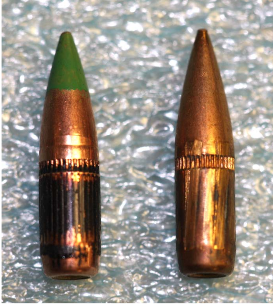
Figure 2. Unfired (left) and soft recovered (right) 5.56-mm M855 projectiles.
