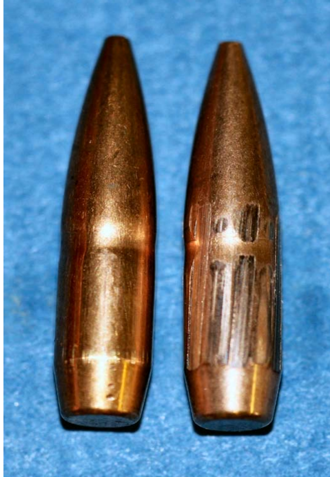
Figure 3. Unfired (left) and soft recovered (right) 0.223 Remington Match projectiles.
