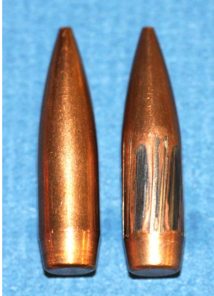
Figure 4. Unfired (left) and soft recovered (right) 7.62-mm M118LR projectiles.
