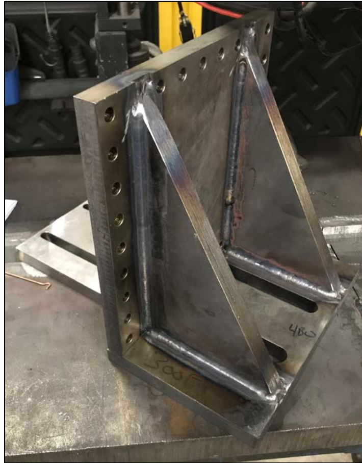
Figure 13. Backplate Support Showing Gussets
