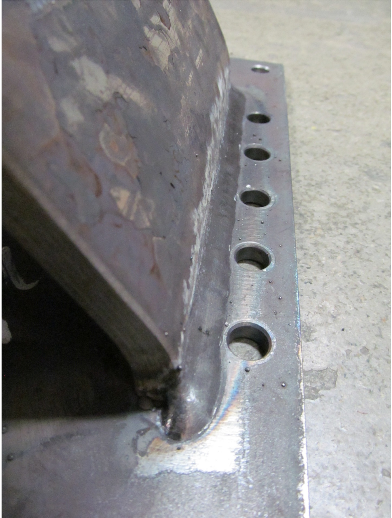
Figure 15. Example Fillet Weld Shown After Testing from the Start End
