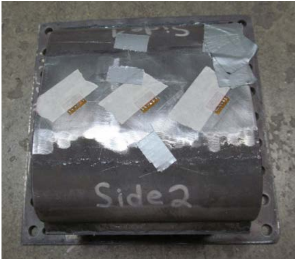
Figure 17. Welded Channel Showing Placement of Strain Gage Strip Rosettes
