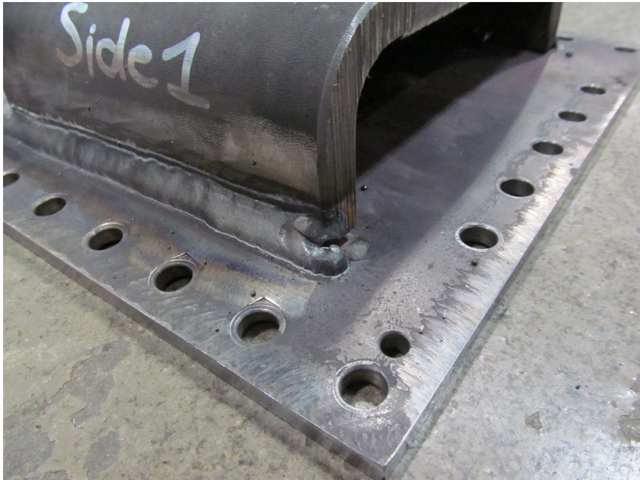
Figure 20. Short Crack Localized on Weld End
