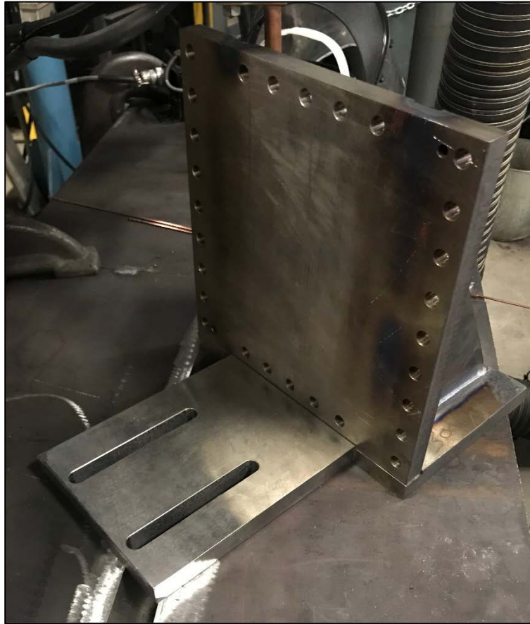
Figure 12. Backplate Support Showing Front Side Where the Backplate Will Be Bolted to the Face
