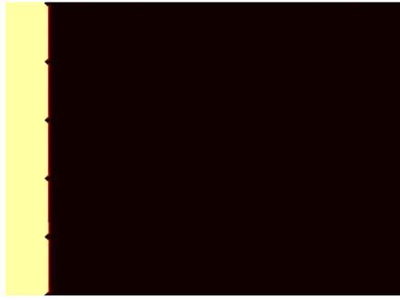
(a) Screen shot taken at time=0 to show the initial disturbed placed at the interface in order to promote the occurrence of viscous fingering
