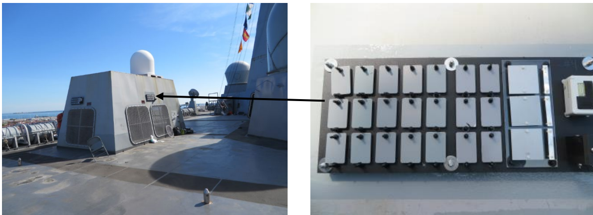
Figure 6 – Exposure rack deployed on an LPD 17 class ship
