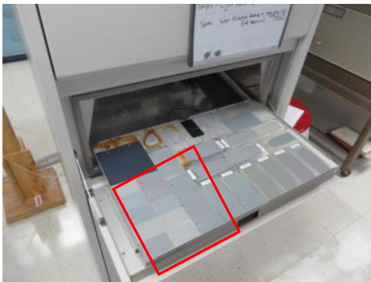
Figure 3 – Test panels in xenon arc test chamber
