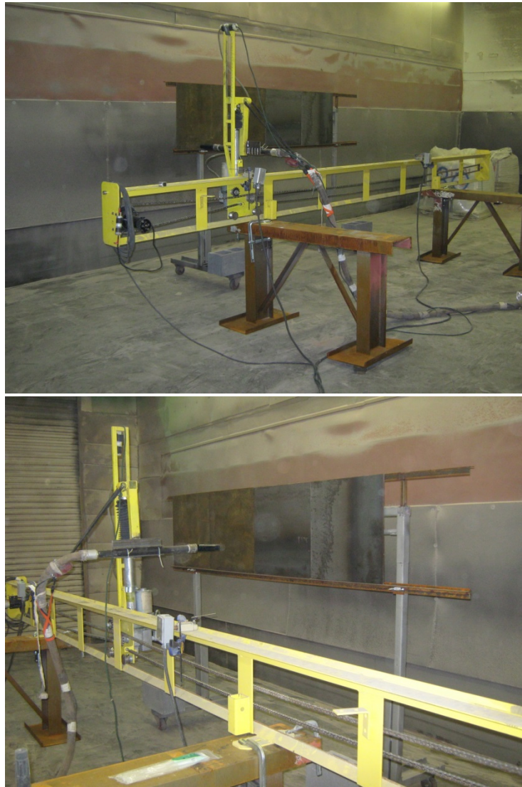
Figure 27 – Semi automated blast nozzle for blasting larger test panels at controlled rates
