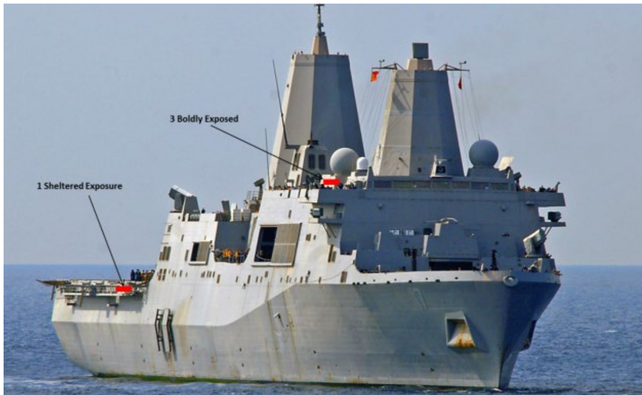
Figure 20 – Exterior locations of exposure racks on an LPD 17 class ship
