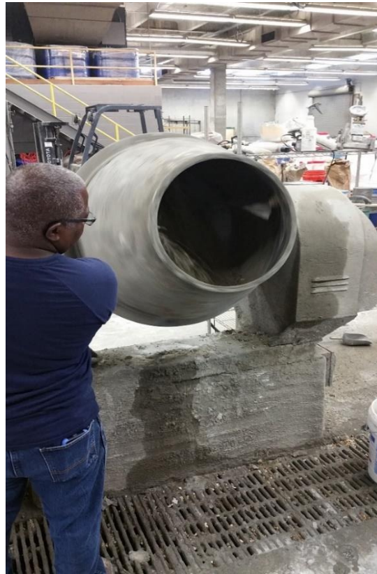
Figure 8. Worthington 3-ft 3 steel drum concrete mixer.
