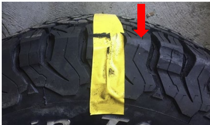
Figure 7. BFG 35 tire with simulated wear ( right side, shown with arrow ).
