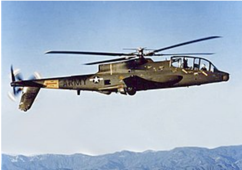
Figure 1.2. Lockheed AH-56A Cheyenne, early attempt at a high-speed attack helicopter that suffered from handling qualities related issues.
