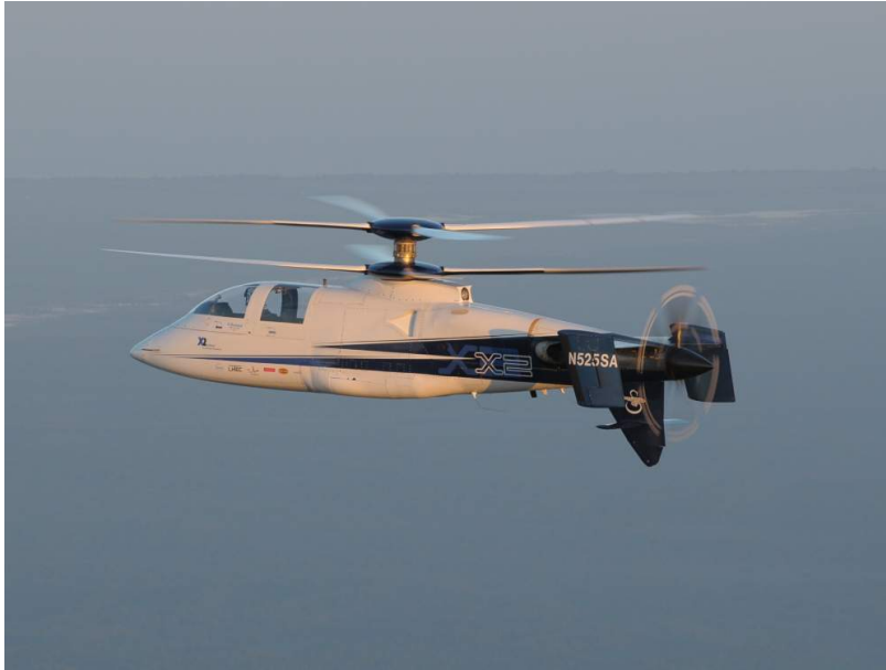
Figure 1.7. Sikorsky Aircraft X2 Technology Demonstrator, continued development of Advancing Blade Concept (ABC).
