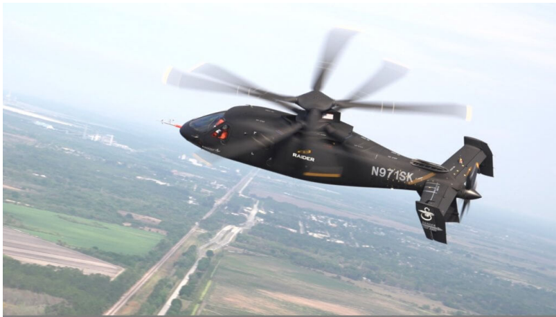
Figure 1.11. Sikorsky S-97 Raider, high-speed scout and attack compound helicopter based on the Advancing Blade Concept (ABC).
