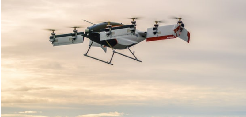
Figure 1.16. Airbus Vahana eVTOL aircraft, eight-propeller tilt-wing demonstrator.
