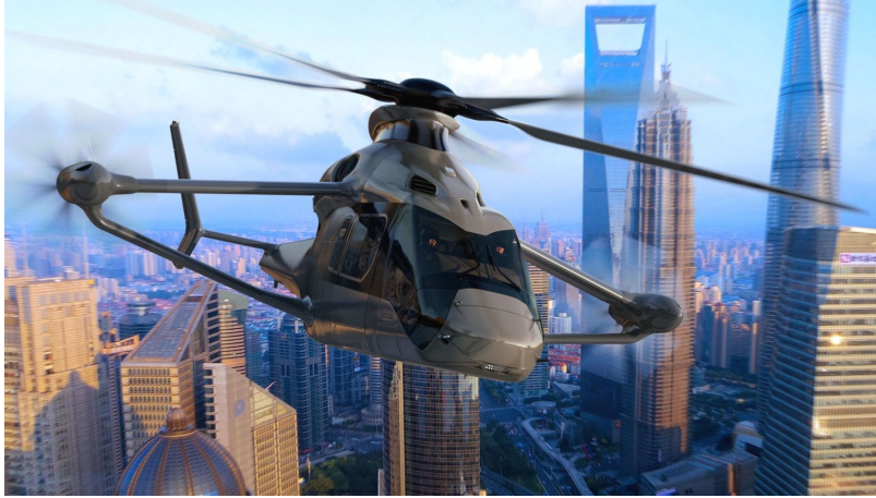
Figure 1.14. Airbus RACER (Rapid and Cost-Effective Rotorcraft), one of two aircraft being developed as part of the Clean Sky 2 Fast Rotorcraft Innovative Aircraft Demonstrator Platform.
