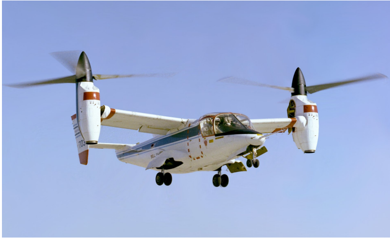
Figure 1.5. Bell XV-15, first experimental tiltrotor to successfully demonstrate high-speed performance.
