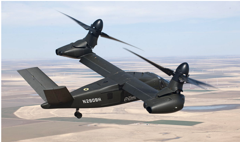
Figure 1.9. Bell V-280 Valor tiltrotor, one of two Joint Multi-Role Technology Demonstrator aircraft.
