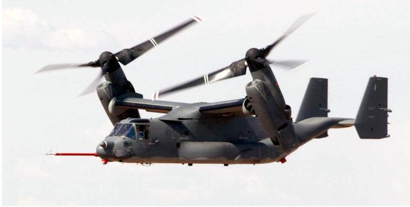
Figure 1.6. Bell Boeing V-22 Osprey, first production tiltrotor aircraft.
