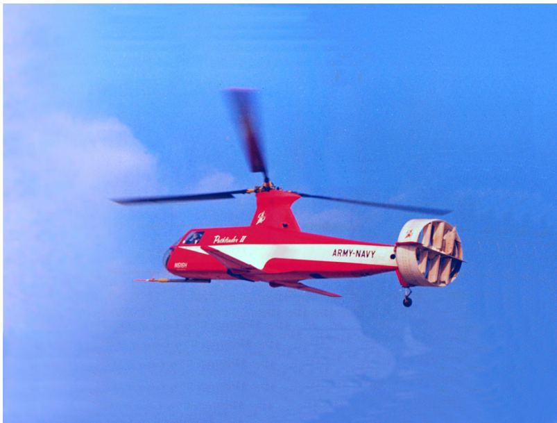
Figure 1.1. Piasecki 16H-1A Pathfinder II, early example of compound rotorcraft.
