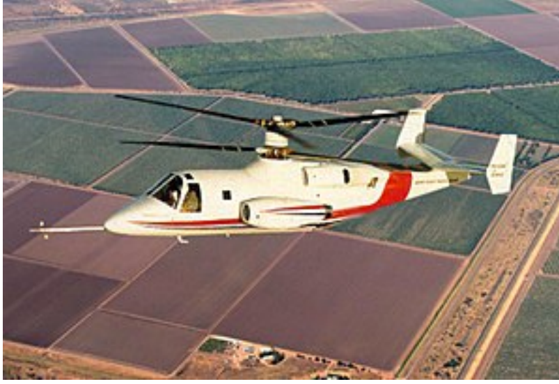
Figure 1.3. Sikorsky Aircraft S-69/XH-59A, successfully demonstrated the Advancing Blade Concept (ABC).
