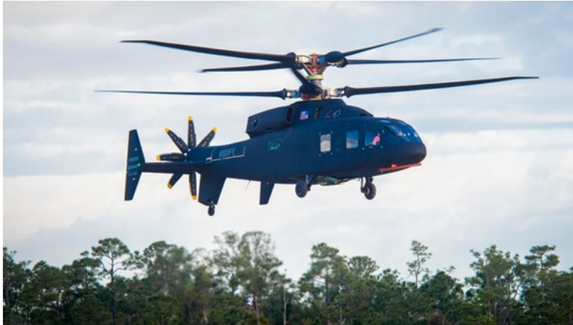
Figure 1.10. Sikorsky Boeing SB-1 Defiant Advancing Blade Concept (ABC) rotorcraft, one of two Joint Multi-Role Technology Demonstrator aircraft.
