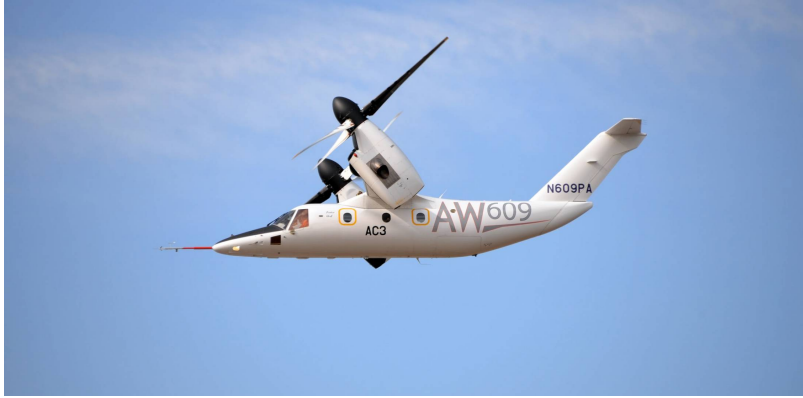
Figure 1.12. Leonardo AW609, aimed to be the first production tiltrotor for civil use.
