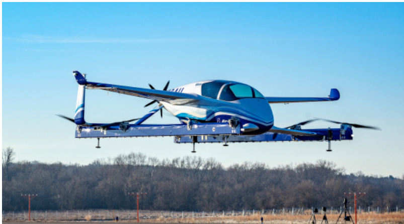
Figure 1.17. Boeing NeXt autonomous eVTOL prototype.
