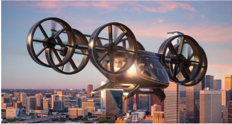
Figure 1.18. Bell Nexus hybrid-electric VTOL aircraft concept.
