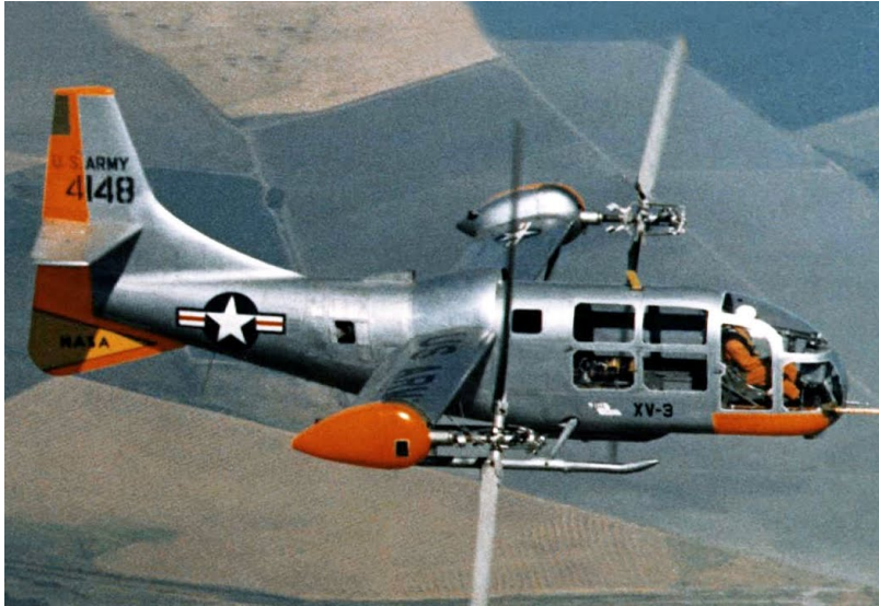
Figure 1.4. Bell XV-3, successfully demonstrated the tiltrotor concept.
