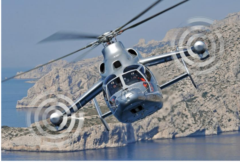
Figure 1.8. Airbus Helicopters (formerly Eurocopter) X 3 , fastest non-jet augmented compound helicopter.
