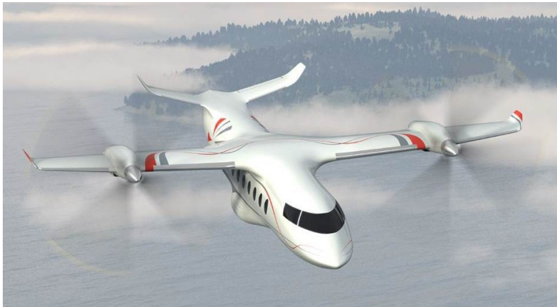
Figure 1.15. Leonardo Next-Generation Civil Tiltrotor, one of two aircraft being developed as part of the Clean Sky 2 Fast Rotorcraft Innovative Aircraft Demonstrator Platform.
