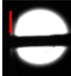
Fig. 2 Individual frame from shot 6, spark gap position indicated by red arrow
