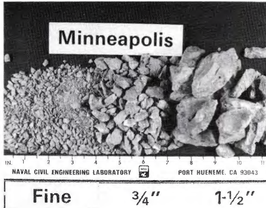
FIGURE 14. PRODUCTS FROM THE CRUSHING OF THE PCC SAMPLE FROM MINNEAPOLIS.
