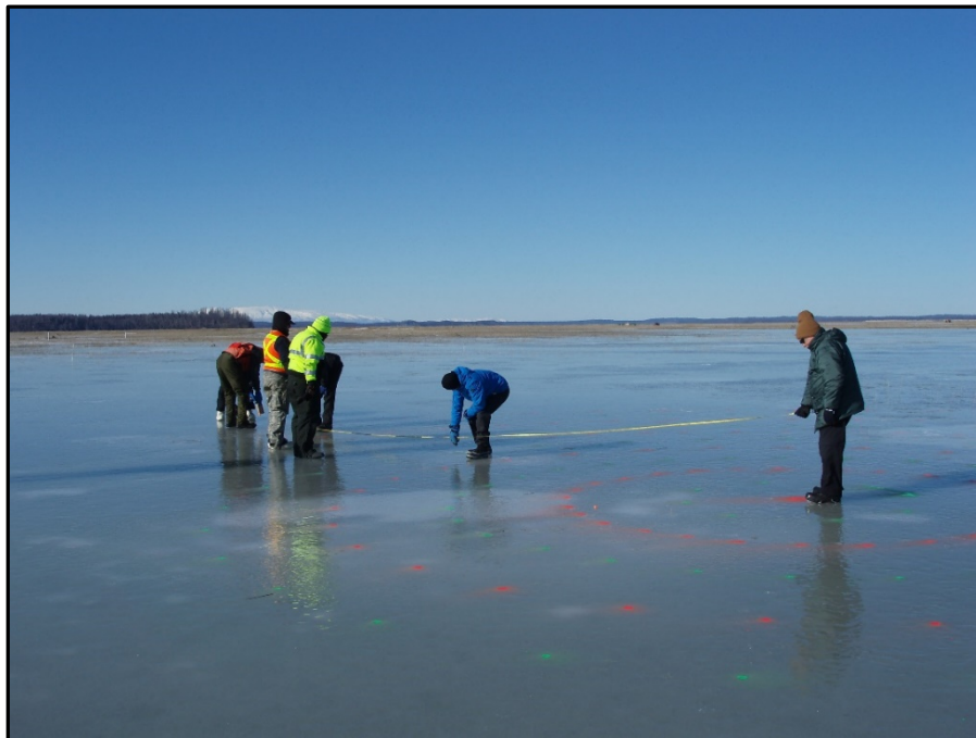
Figure 2. Marking 1 m annuli around the detonation point. Rings were marked in alternating colors.
