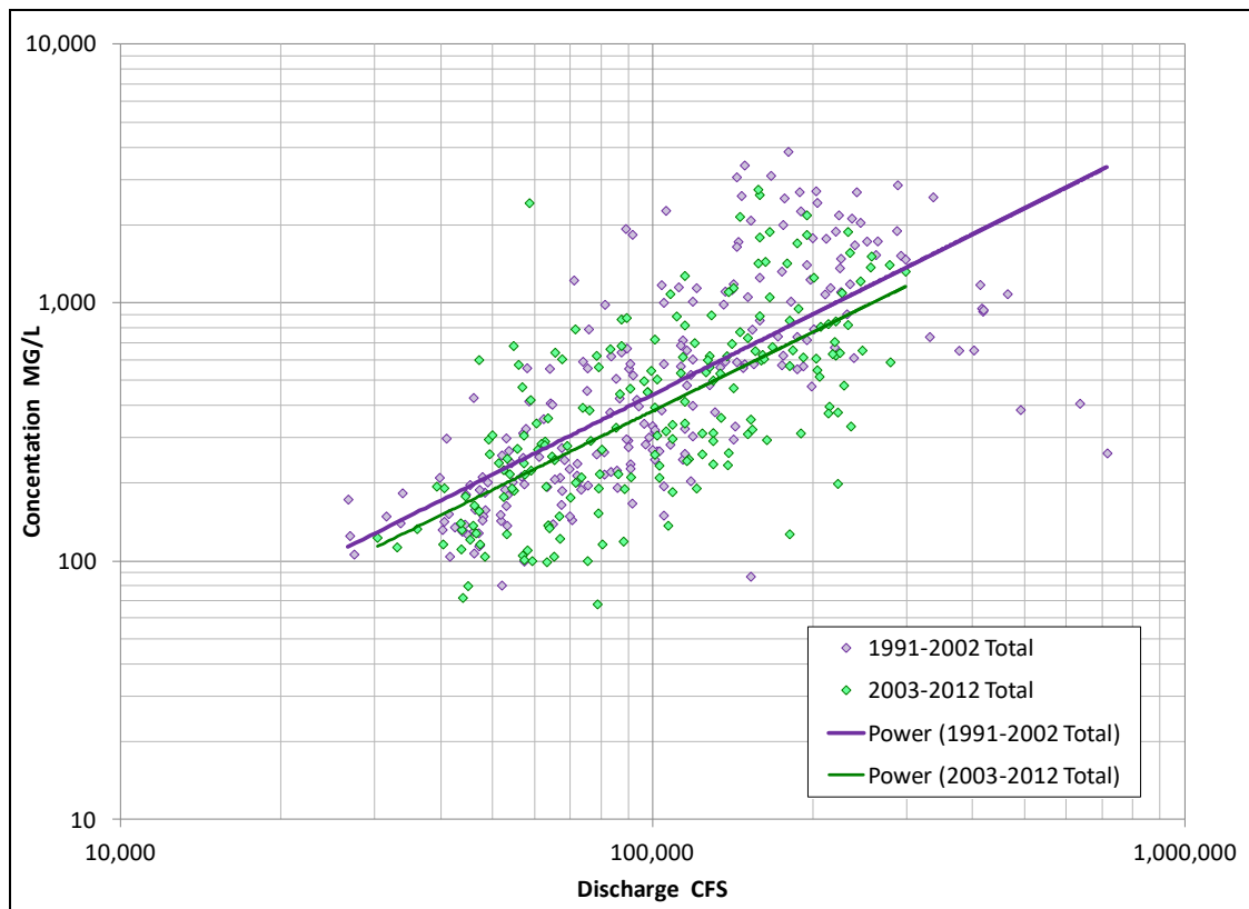
Figure 135. Measured total suspended sediment concentration, at Hermann.
