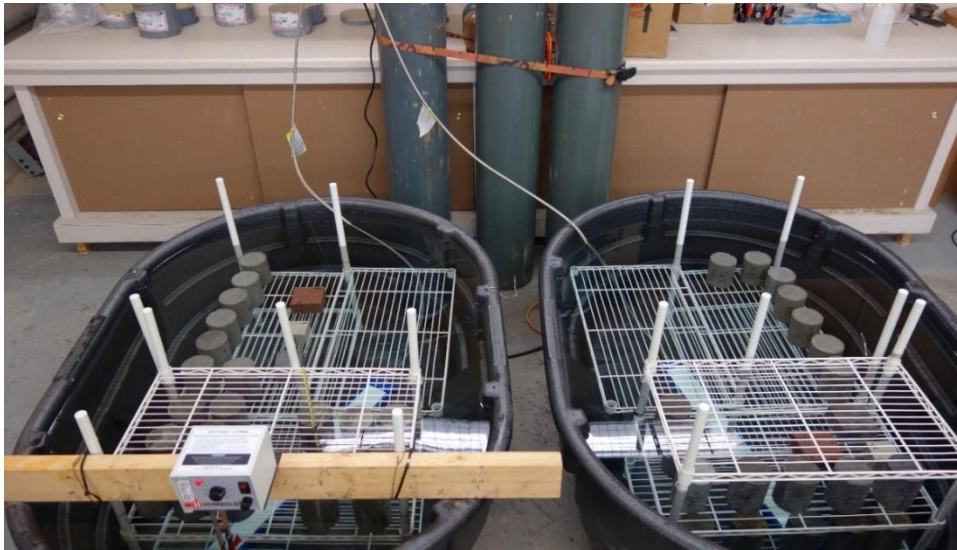
Figure 2. Carbonation exposure system consisting of two tanks with CO 2 injection systems and heater to control tank two temperature.
