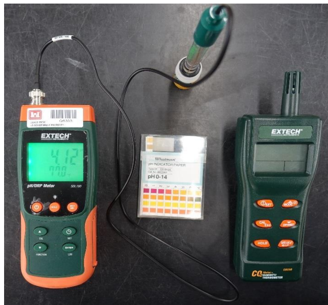
Figure 3. Carbonation Extech digital meters (pH, temperature, carbon dioxide, and relative humidity).
