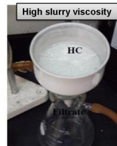
Filtration of ZnO and Al 2 O 3
