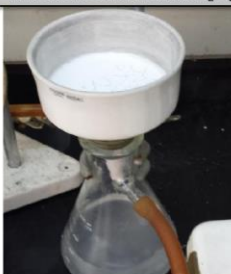
Filtration of ZnO and Al 2 O 3
