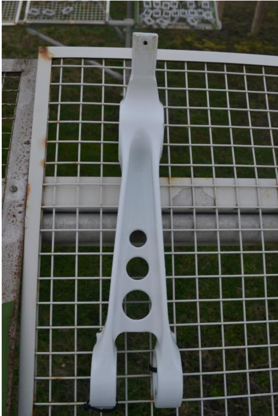
Figure 165: Painted Cd Plated Drag Brace (3/2/2016)
