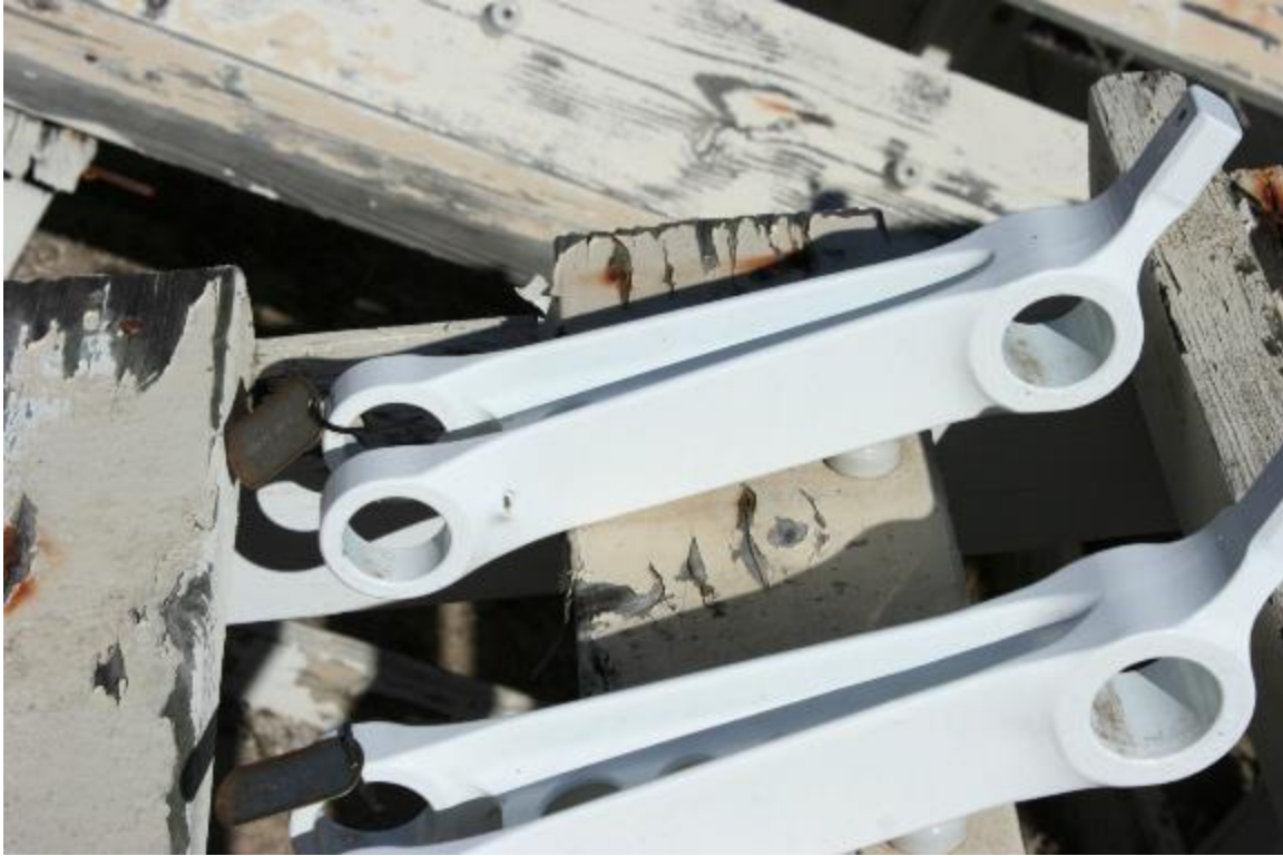
Figure 137: Cd (Far) and LHE Zn-Ni (Near) Painted Drag Braces (11/4/2015)
