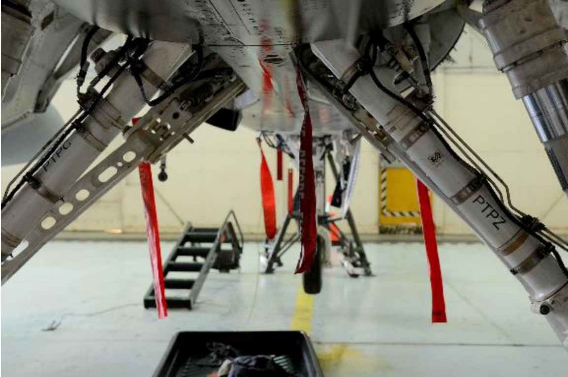
Figure 78: LHE Zn-Ni and Cd plated components on installation (12/16/2014)
