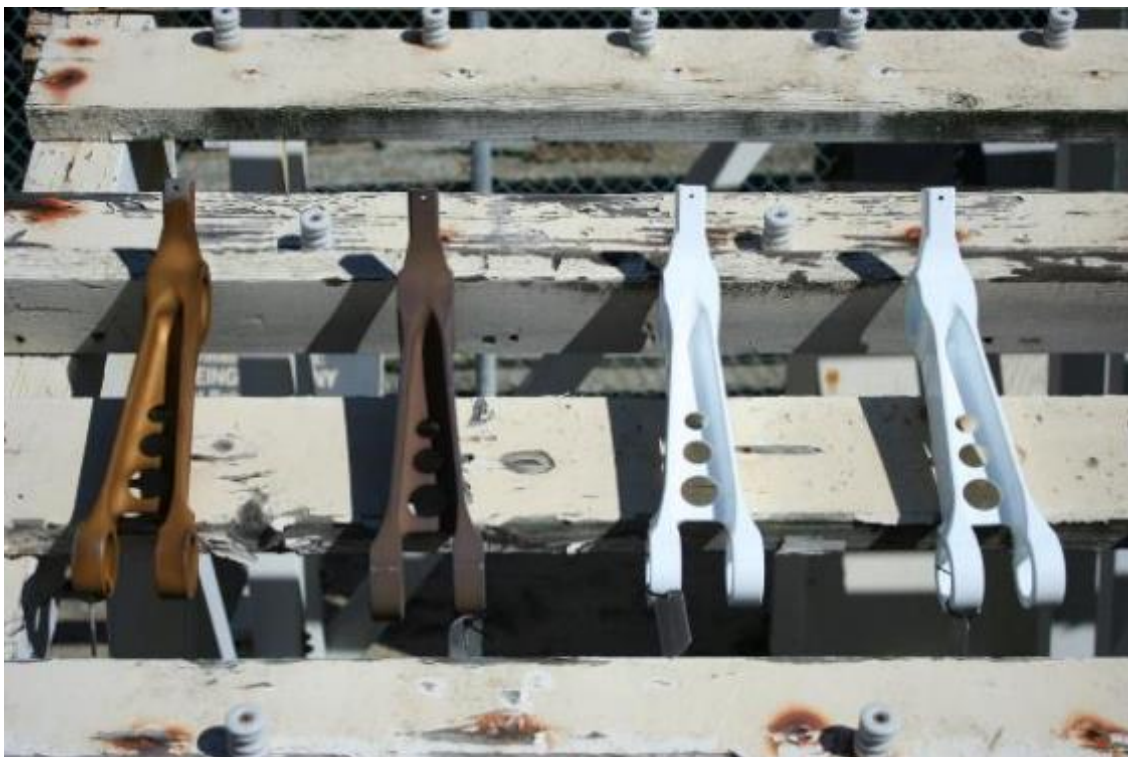
Figure 93: Corrosion Test Subjects on Installation (Cd, LHE Zn-Ni, Cd Painted, LHE Zn-Ni Painted) (11/3/2014)
