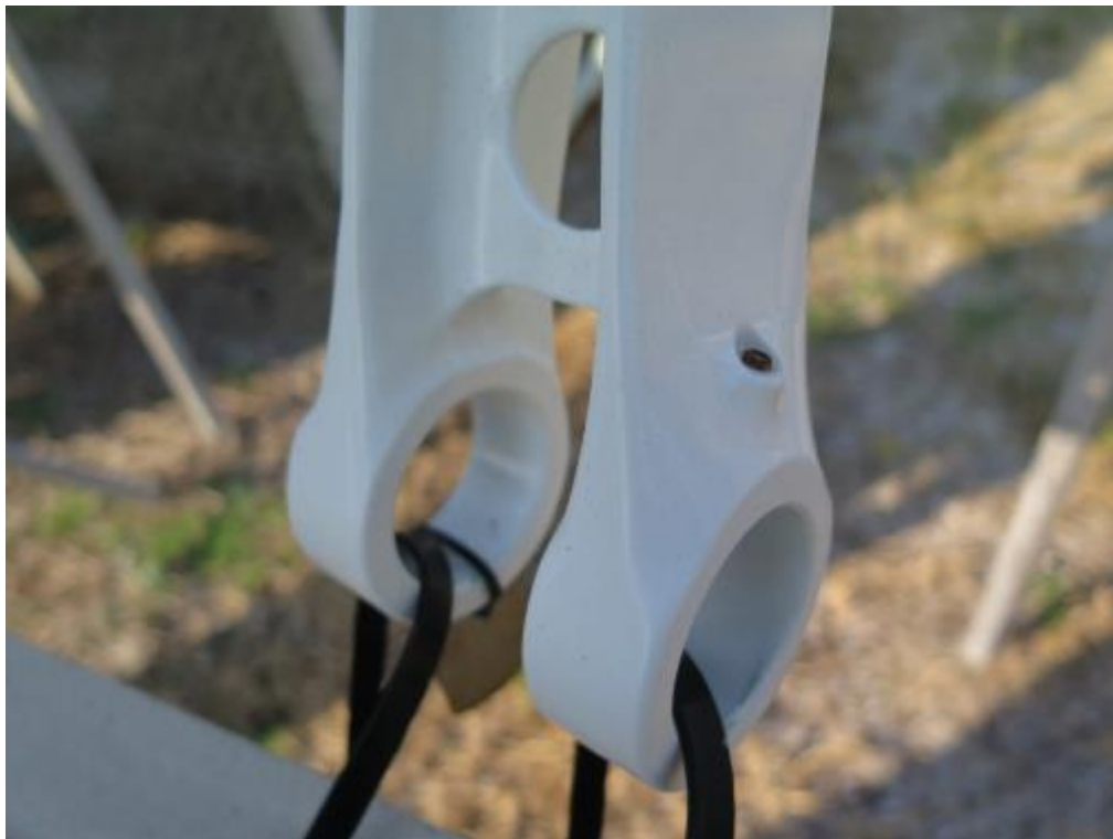
Figure 109: Painted Cd Plated Drag Brace (8/26/2015)
