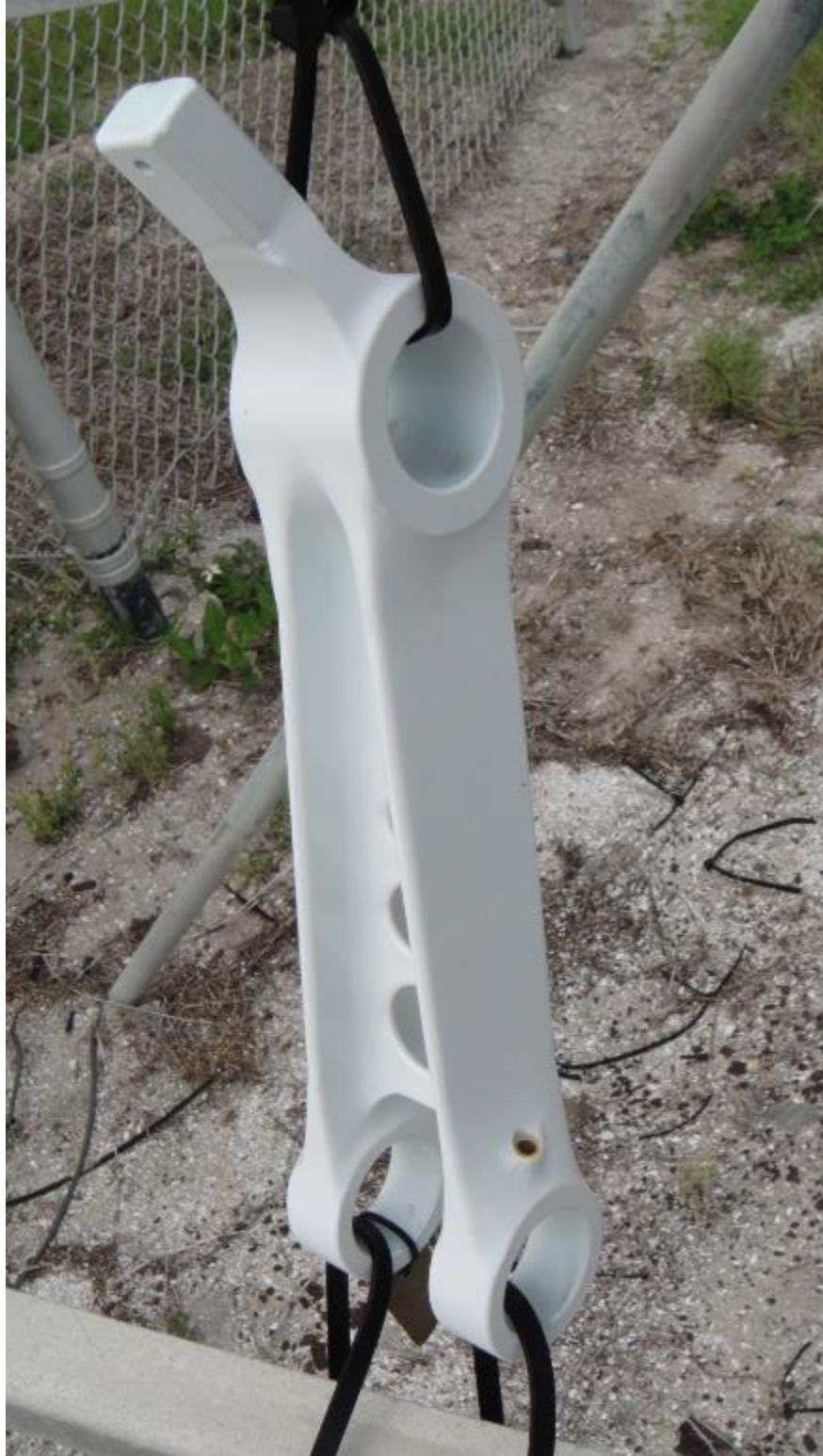
Figure 121: Painted Cd Plated Drag Brace (8/26/2016)
