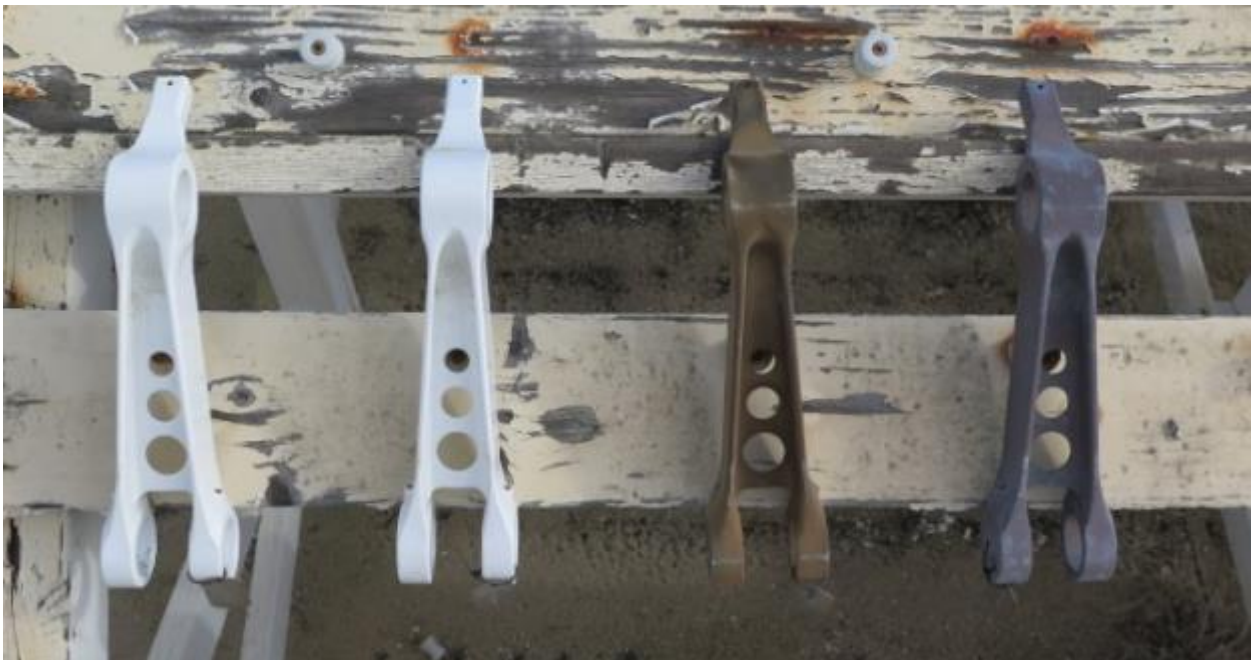
Figure 142: Painted Cd, Painted LHE Zn-Ni, Cd, and LHE Zn-Ni Plated Drag Braces (1/18/2017)
