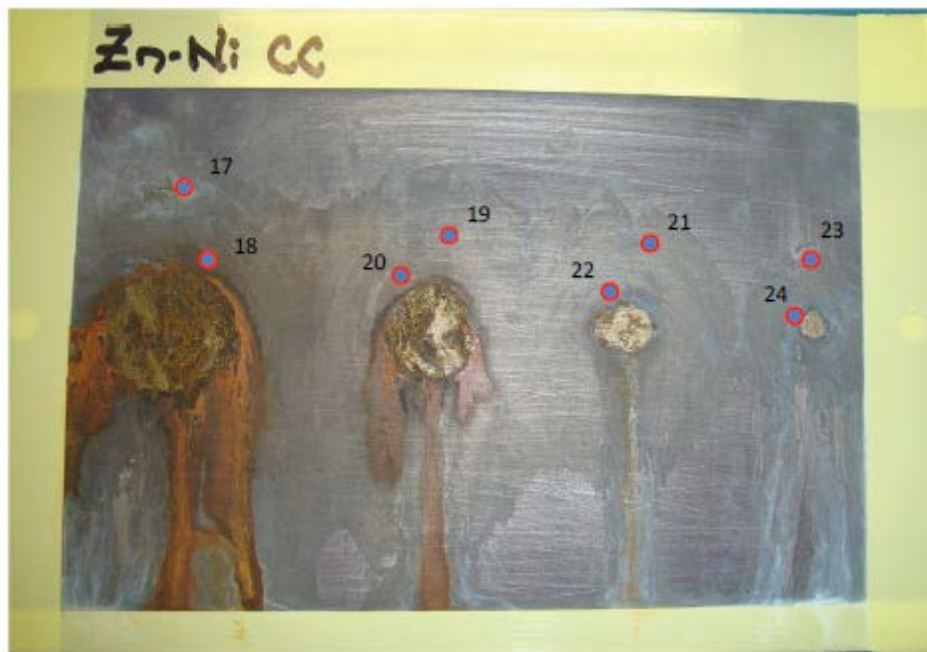
Figure 39: LHE Zn-Ni with Conversion Coat XRF Analysis Locations
