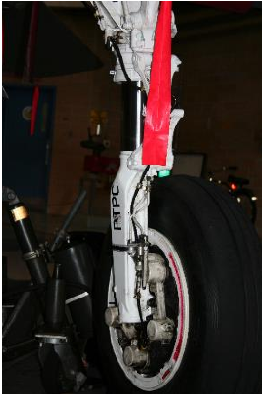
Figure 54: Installation of Cd Plated Component
