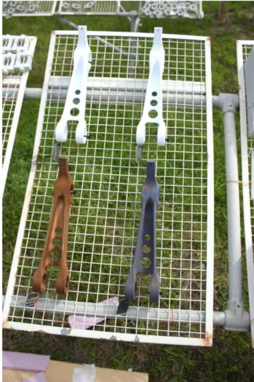
Figure 95: Cd and LHE Zn-Ni Plated Test Components at Whidbey Island on Installation (Top Left Cd Painted, Right LHE Zn-Ni Painted, Bottom Left Cd, Right LHE Zn-Ni) (05/14/2014)
