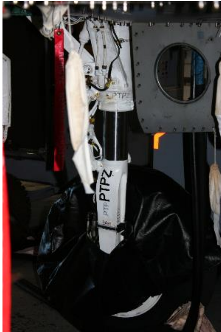
Figure 59: Installation of LHE Zn-Ni Plated Component
