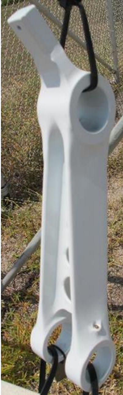
Figure 99: Painted Cd Plated Drag Brace (7/13/2015)
