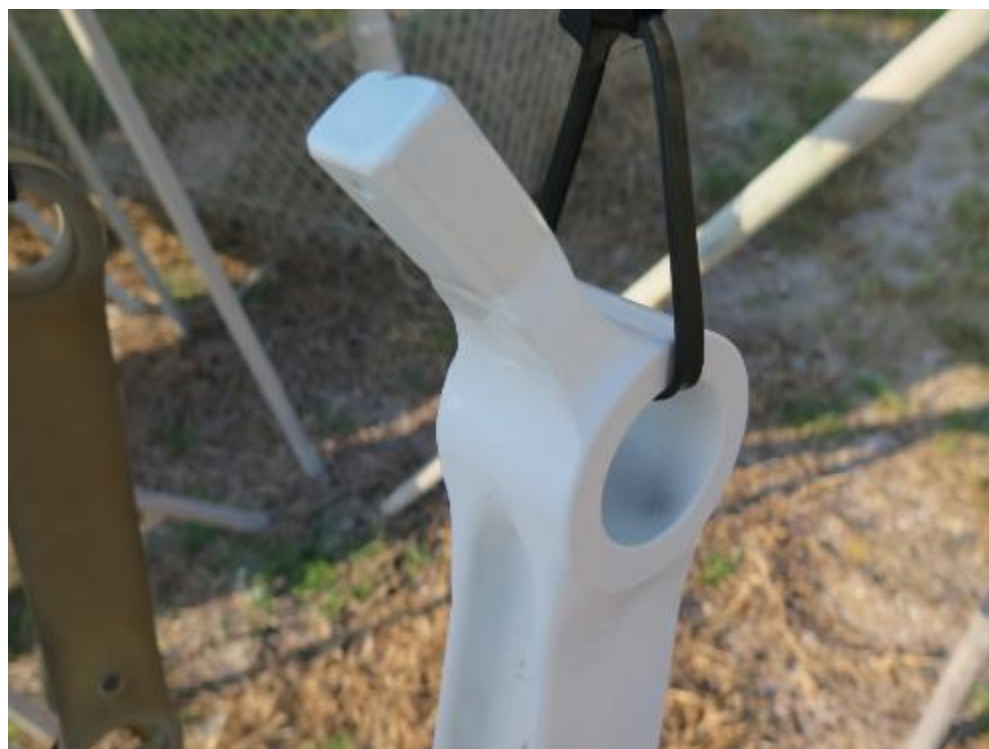
Figure 107: Painted Cd Plated Drag Brace (8/26/2015)
