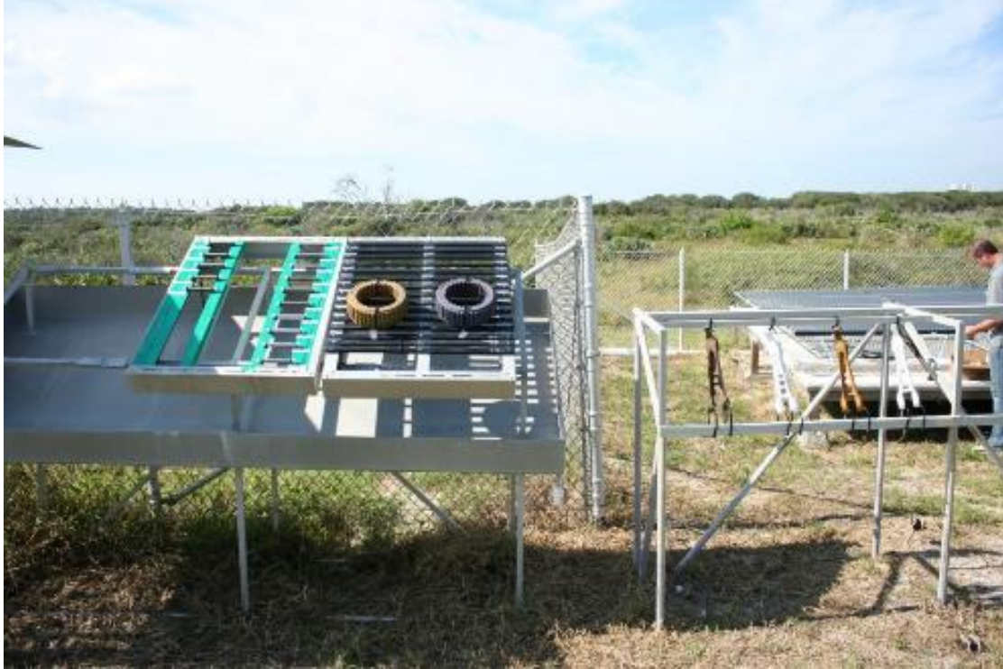
Figure 89: Corrosion Testing Components at NASA Atmospheric Corrosion Test Site Install (10/22/2014)
