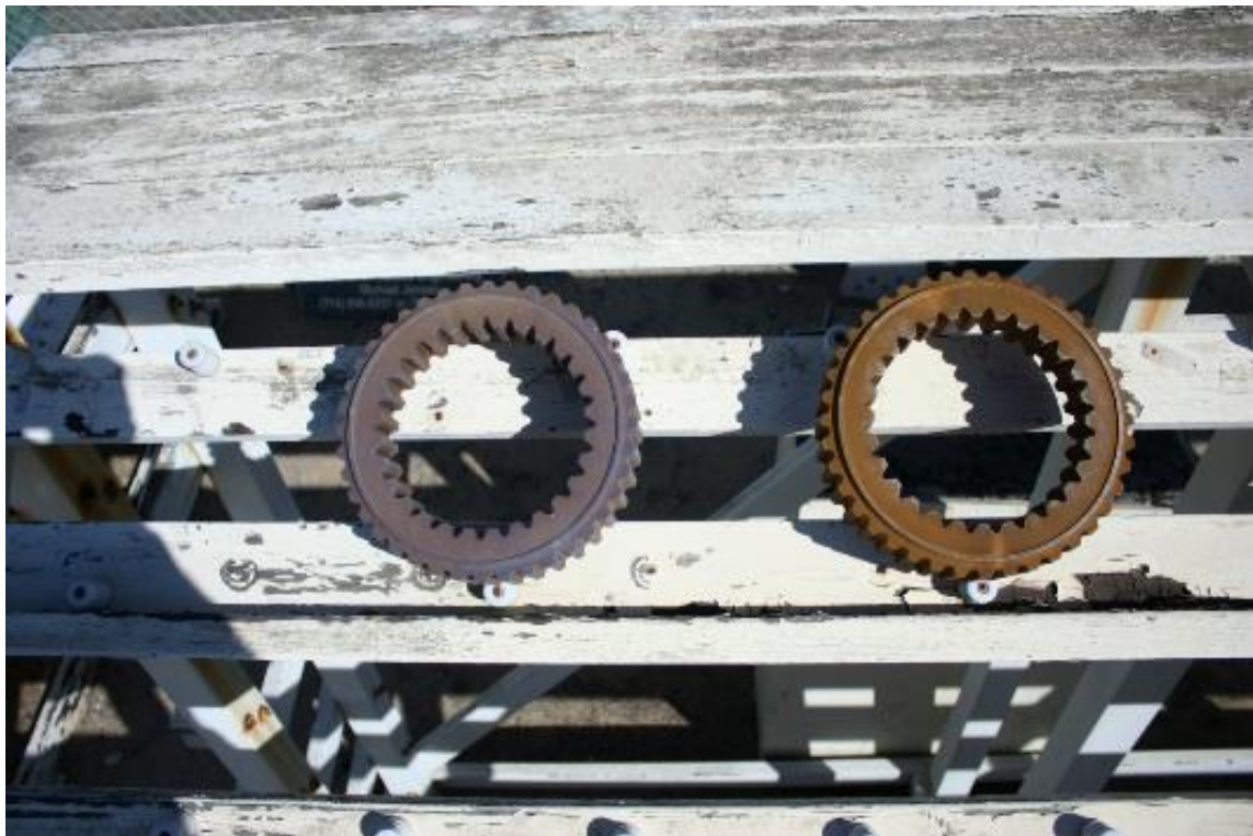
Figure 92: Corrosion Test Subjects on Installation LHE Zn-Ni Left, Cd Right (11/3/2014)
