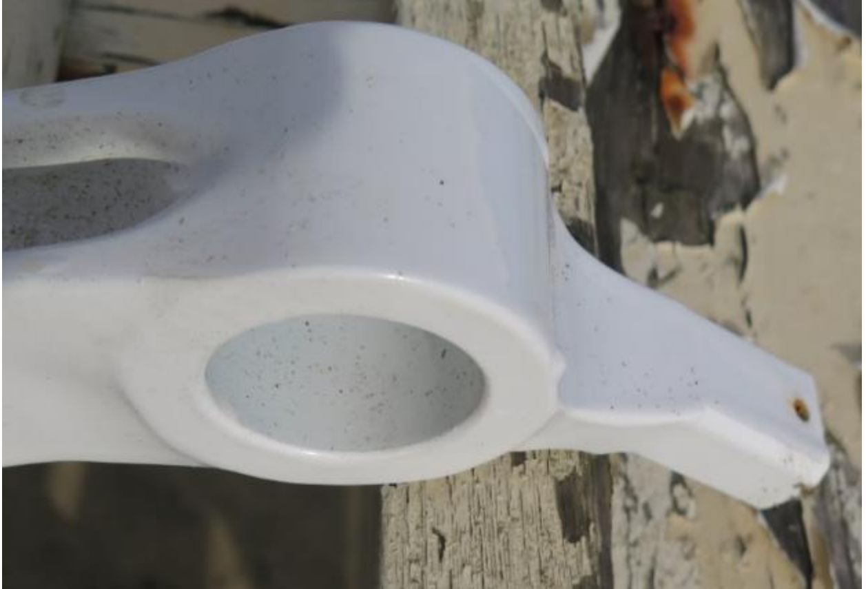
Figure 146: Painted Cd Plated Drag Brace (1/18/2017)
