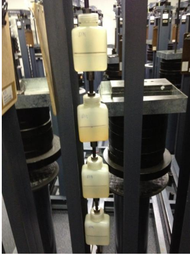
Figure 45:Re-embrittlement Test Setup
