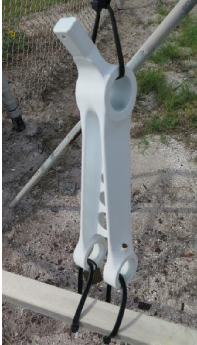
Figure 126: Painted Cd Plated Drag Brace (4/6/2017)
