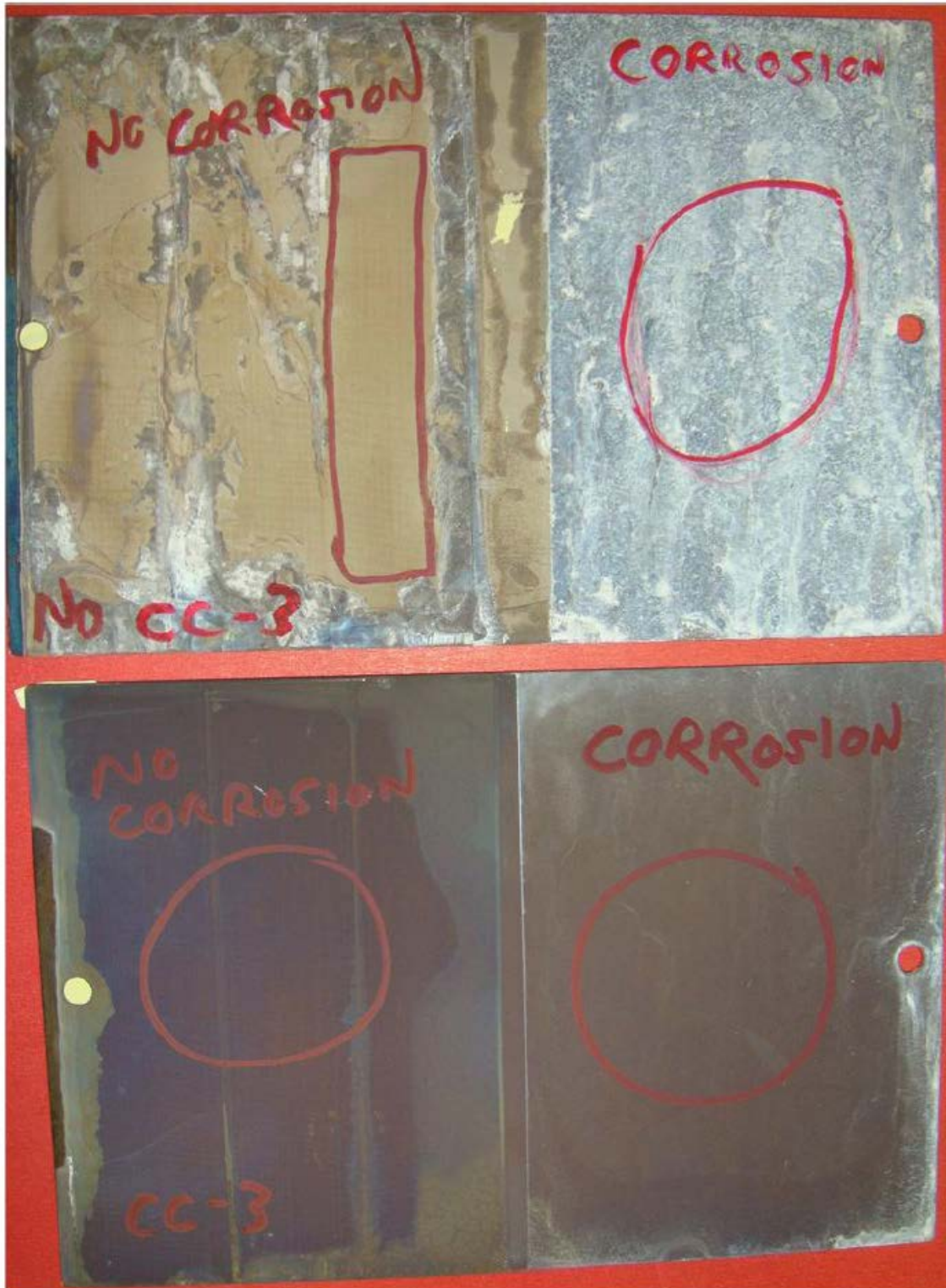
Figure 24: Corroded and Un-corroded areas of LHE Zn-Ni Panes CC-3 (bottom) and NCC-3 (top) after 4 Weeks in ASTM B117 Salt Spray
