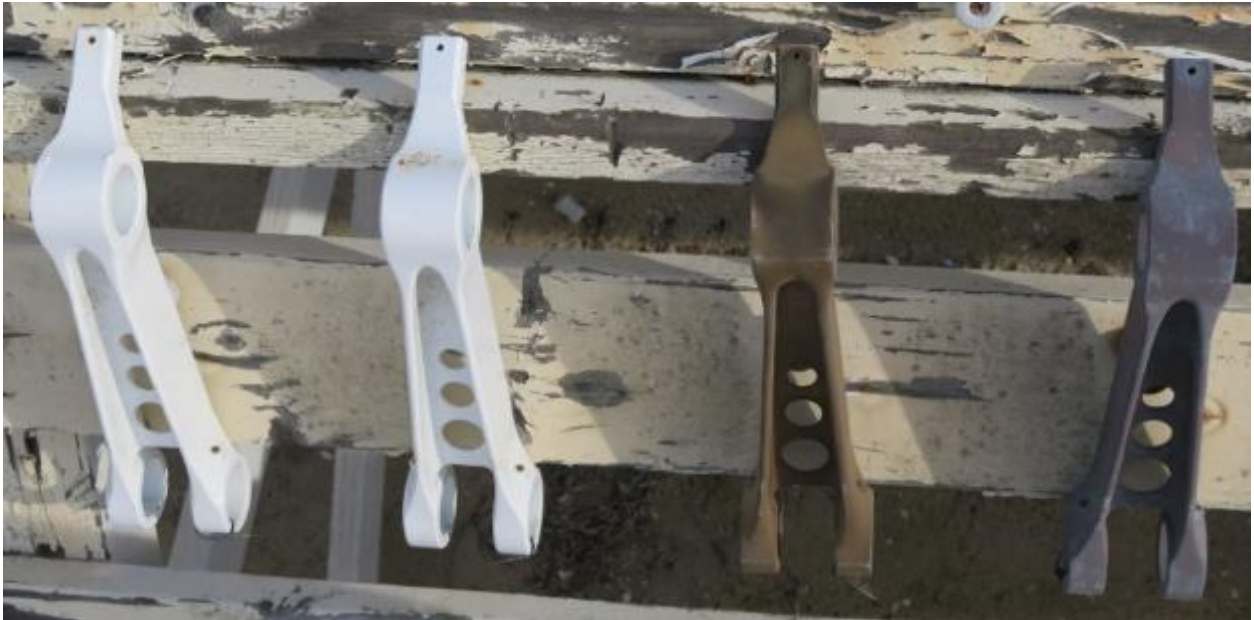
Figure 141: Painted Cd, Painted LHE Zn-Ni, Cd, and LHE Zn-Ni Plated Drag Braces (1/18/2017)
