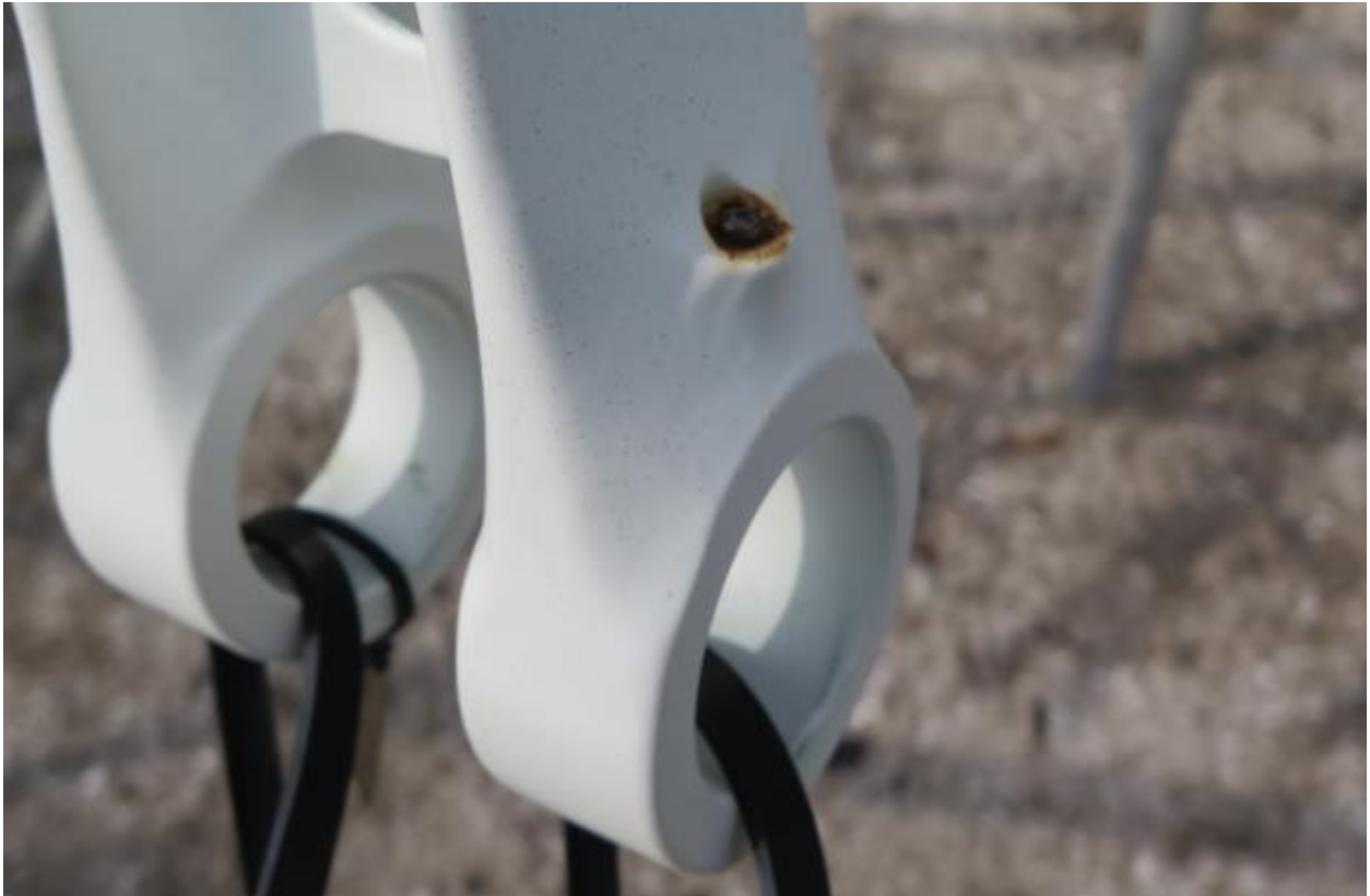
Figure 127: Painted Cd Plated Drag Brace (4/6/2017)
