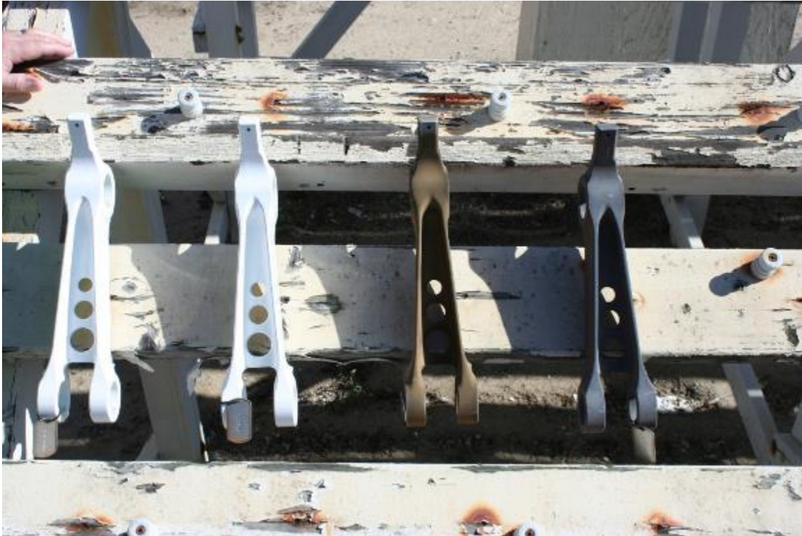
Figure 135: El Segundo Corrosion Drag Braces (Cd Painted, LHE Zn-Ni Painted, Cd, LHE Zn-Ni) (11/4/2015)
