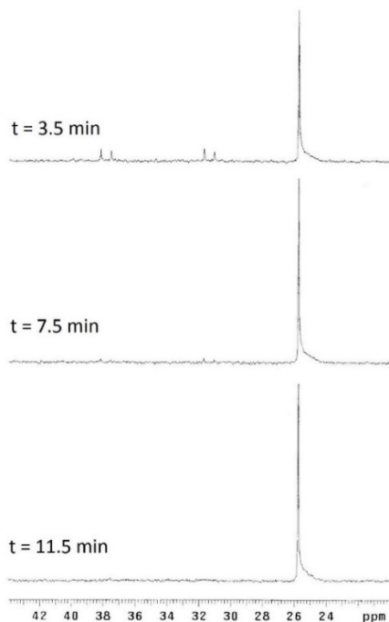
Figure 165. Select 31 P NMR spectra obtained for 2.6 μL GD added to 2.6 mg UiO-66-NH 2 in 0.75 mL 0.5 M EM buffer.
