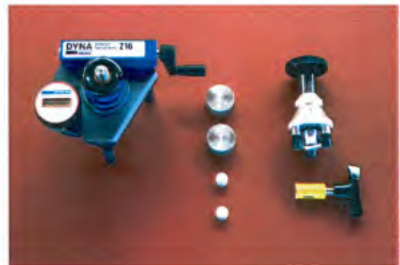
Commercially available portable adhesion testers: Dyna Tester and Elcometer™.
