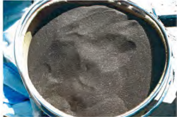
#60 mesh emery ore non-skid (aluminum oxide).
