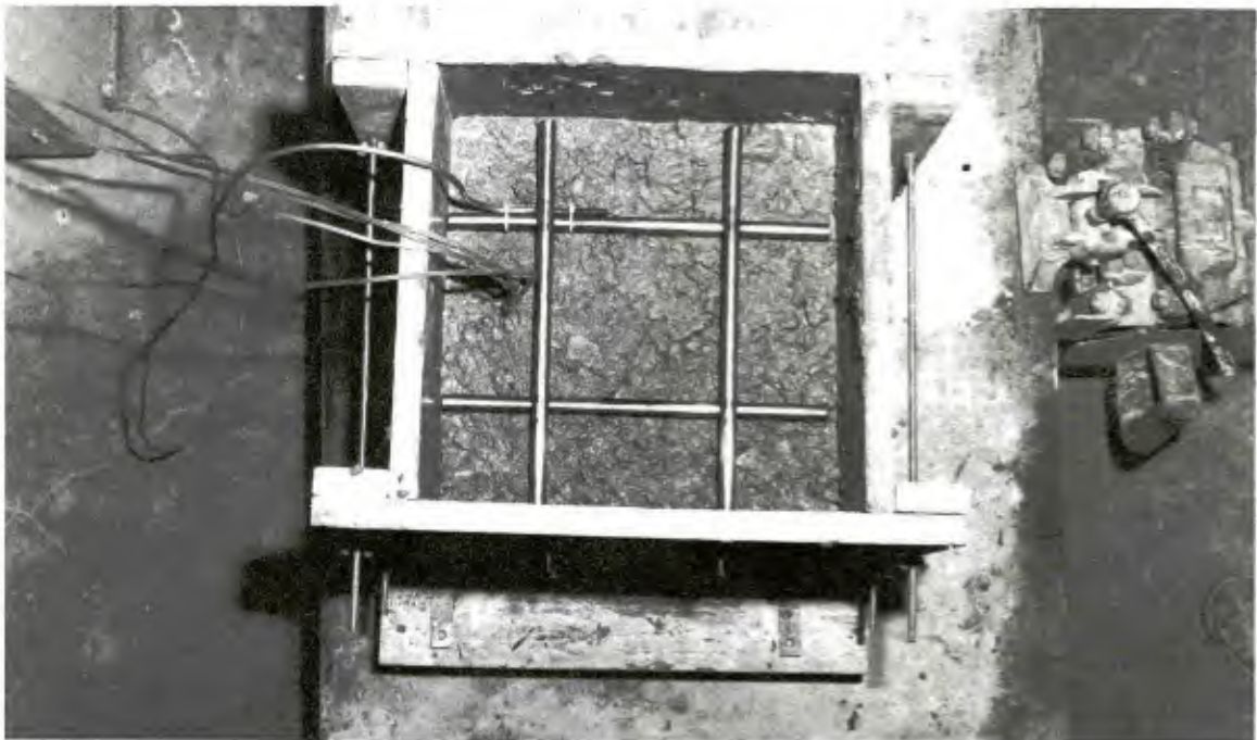
Figure 2. Typical 6 by 6-inch welded wire fabric instrumented with weldable strain gage.
