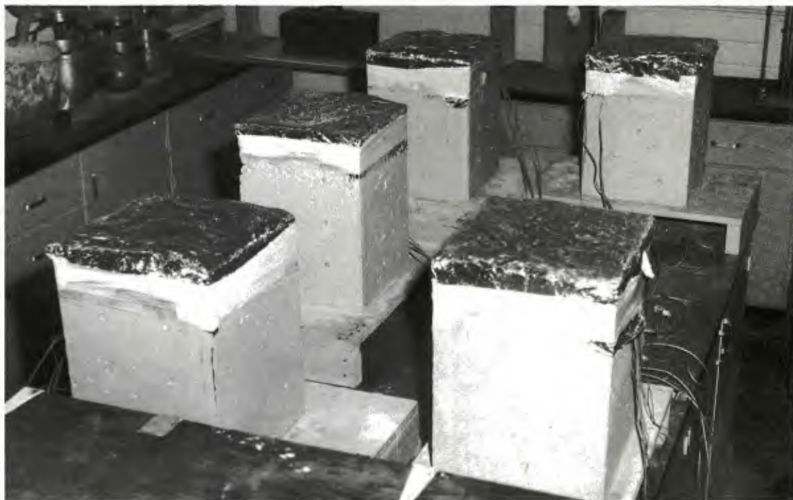
Figure 4. Prismatic slab-type specimens being cured.
