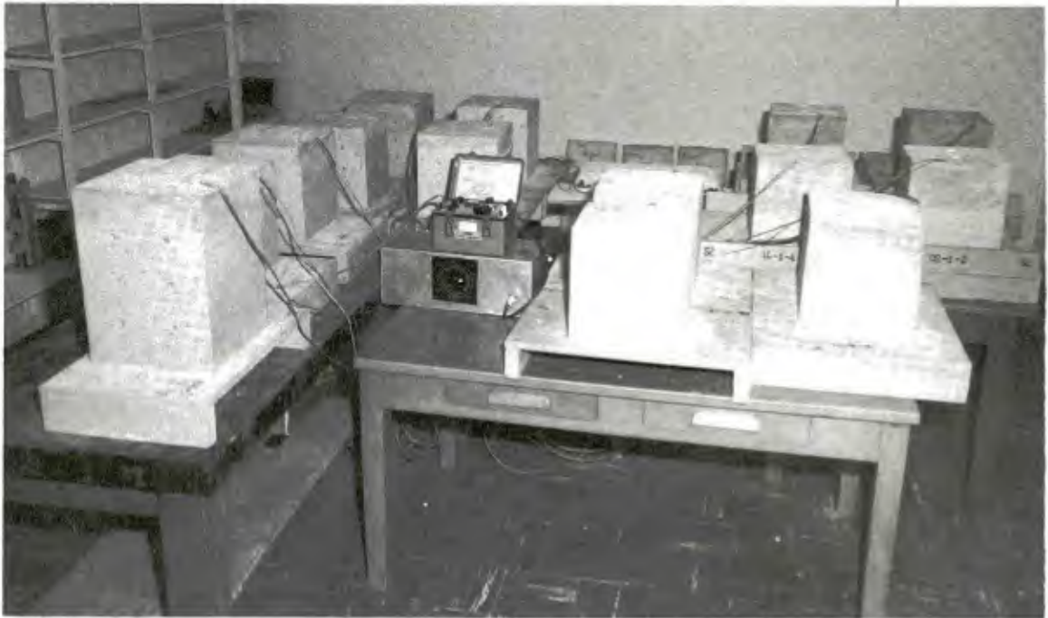
Figure 1. Prismatic slab-type specimens in drying environment.
