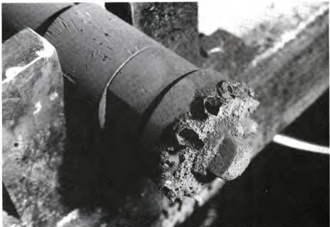
b. After 18 hours of firing no. 6 fuel oil.
