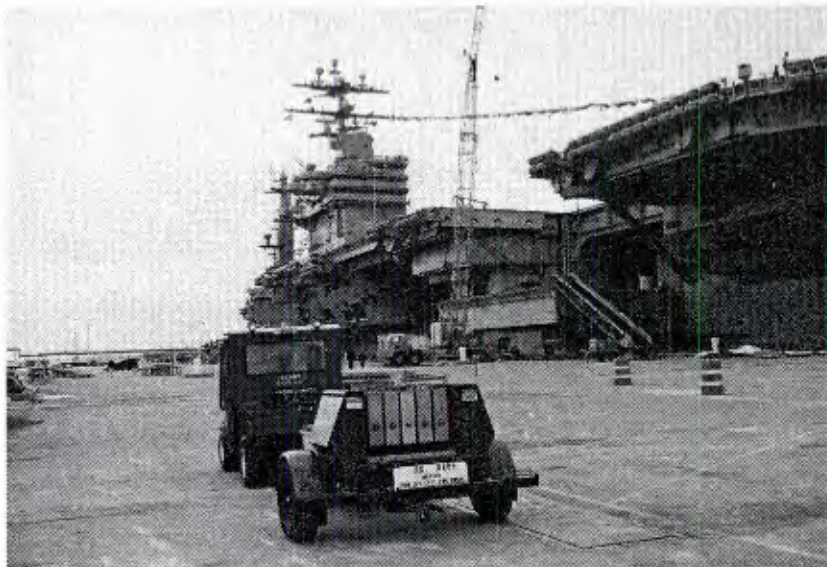
Figure 5. Falling weight deflectometer used to load test pier 11.
