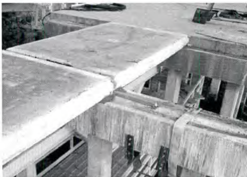
Figure B17. Slab tests being prepared on the AWTTS.
