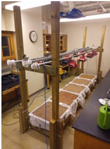
Figure 2: Shows the lab setup of the 5 KRC soils. The soils in order from bottom left to top right: 2NS, Stability, Rink, Coarse, and Fine. Above each bin are two 500-Watt work lights, and the middle bar is the track the hyperspectral camera is moved along.
