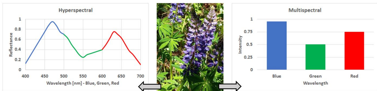
Figure 3: Shows the difference in both the number and width of bands for hyperspectral (Left) and multispectral (Right) imaging.
