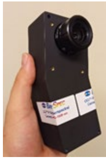
Figure 5: Shows the BaySpec hyperspectral camera used for recording these values. The range of camera is from 400 – 1000 nm.
